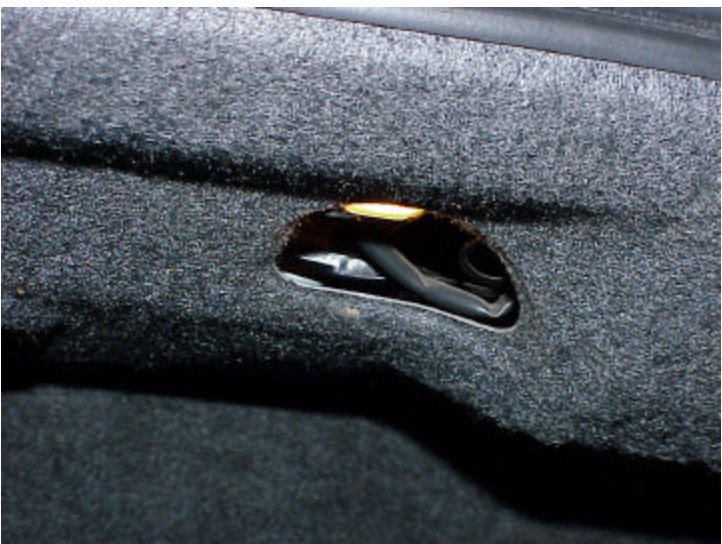
Trunk Room Light (12V – 5W)
