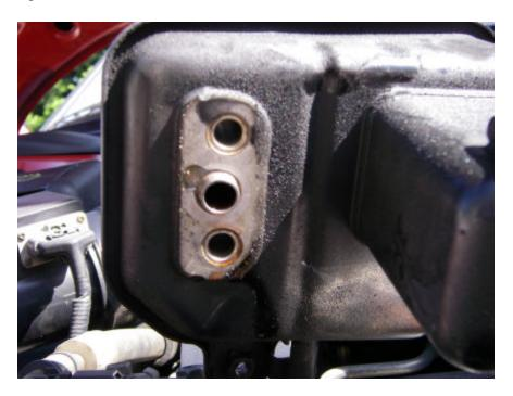
The nipple that the O-ring fits over is seen in the center of the picture. There are 2 other holes, located on the upper and lower side of it. The part number for it is **062610110**, or the actual size is listed on the first page. Once the O-ring is put on, the tank can be put back onto the pump.
