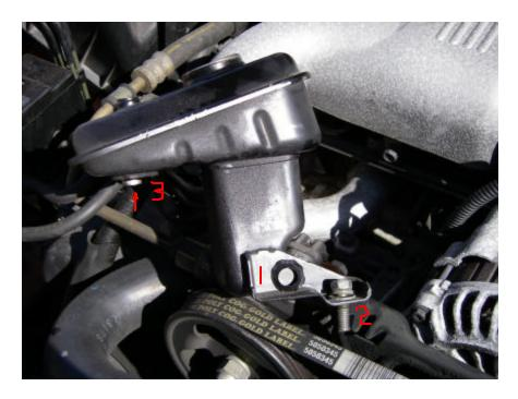
The tank assembly has been lifted off of the pump and the O-ring is ready to be replaced. You can see the old flat O-ring in the center of the picture (1) and the bolt still through the mounting piece (2). The short nipple that the O-ring is on can also be seen (3).
