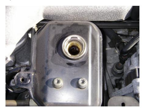
Put the cleaned screen into the tank, and fill it with **Dexron III Transmission Fluid** to the full line on the cap dip stick. It usually will take about 14 to 16 ounces of fluid. There is a mark on it that shows the proper level. Put the cap back on after it is full.
