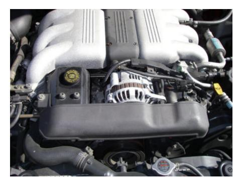
Slide the belt cover back onto the mount piece and then tighten the two 10 mm bolts that hold it on.
