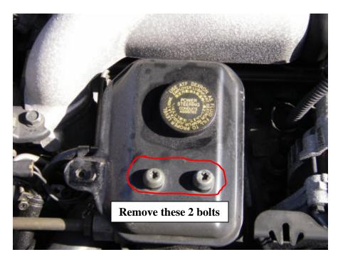
Remove the two (2) Torx head bolts which are size T-40. There is another bolt that needs to be removed, so don't try to remove the tank yet.
