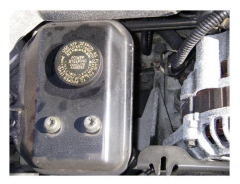
Once the tank is put back onto the pump, start the Torx head bolts (T-40), and then the hex head bolt (12 mm) before tightening.
