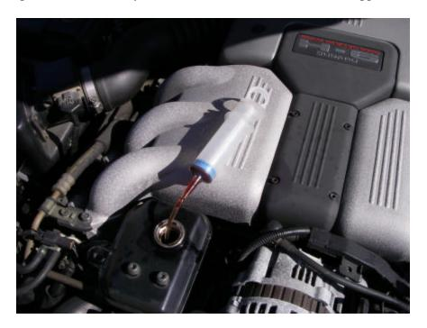
To drain the fluid from the tank, use a syringe or turkey baster. A short piece of tube has been added to this syringe to make it easier to get to the bottom and remove all of the fluid. When full, you will remove approximately 16 ounces of transmission fluid which can be put into a plastic bottle for proper disposal. This needs to be done so that the fluid will not spill onto the engine when the tank is removed from the pump.
