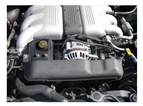
You will need to remove the belt cover which partially covers the tank itself. Do this by removing the two 10 mm bolts on each side of the cover. Be sure to slide the cover forward before lifting up so you will not break it.
