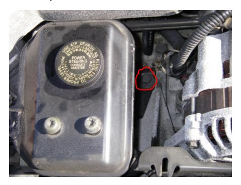
Remove the 12 mm hex bolt next. You will need an extension to reach the bolt. This will allow the tank to be pulled up and rotate to the right to get to where the O-ring is. You can lift the tank and the bolt at the same time so it is not dropped. It will still be connected by some hoses, but you will not need to remove them.
