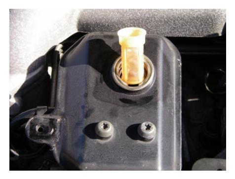
Remove the cap and pull out the screen so the fluid can be taken out. To take it out, put your finger into the screen and then pull it out. You may want to clean it if there is material trapped in it.
