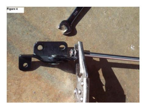
6. Install the upper bolt to the strut by tapping it, and then install the lower strut bracket. Repeat all of the steps for the other bracket which should complete the project.
