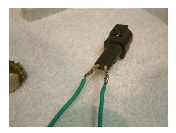
Shrink wrap is then applied to the soldered connections.
