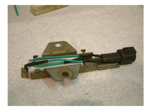
Fold the tabs down to hold the resistor in place. The new resistor is a bit smaller than the old one, but it seems to be held as well as the old one. Note that the forward-most tabs are bent down a little bit further than they used to be.
