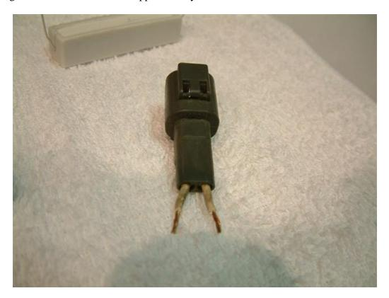
The next step is to solder some new wires to it and it will be helpful to use longer wires than necessary. If this should have to be re-repaired, there will be enough wire for the job, and shrink-wrap can be used instead of electrical tape over the soldered connections.
