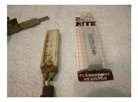
Here is another picture of the old and new resistor. Note the different types of wires attached to both.
