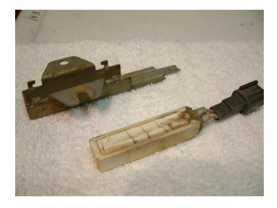
You can see that the old resistor is shows extreme wear. When this resistor was checked with a meter, it showed an open connection!
