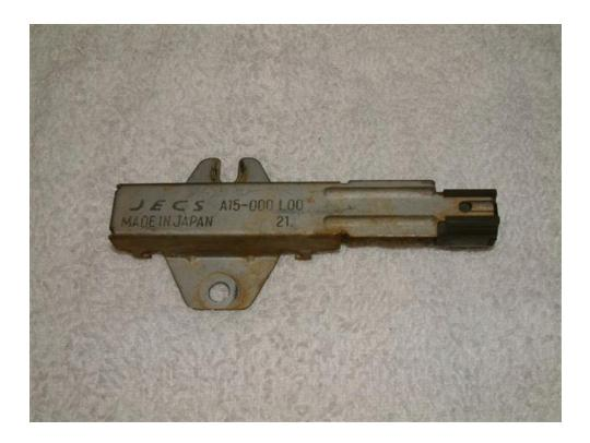
Use a pair of pliers to bend the tabs back and remove the resistor from the bracket.
