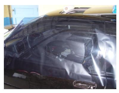
Cut the film so that it lines up with the inside edge of the glass (the clear part). It's OK to leave some additional tint at the bottom, since this part will go below the door panel on the inside of the window.
