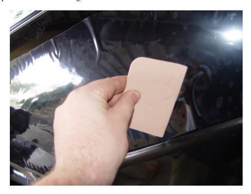
These lines will not smooth out just by using the bondo knife. You'll need to heat them up. Apply some heat to them, one at a time, with the heat gun, and smooth them out with a bunched up paper towel. This is the most difficult part of the process, so take your time. It takes a while to figure out exactly how much heat to apply. This is still on the outside of the window to get the proper shape. The tint will be applied to the inside in the next couple of steps.
