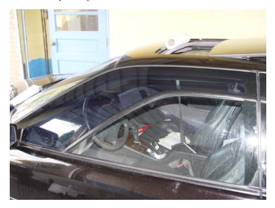
It would be best to install tint in a clean enclosed environment to eliminate particles from getting between the tint and the window. Windows should not be rolled down for several days after application.
