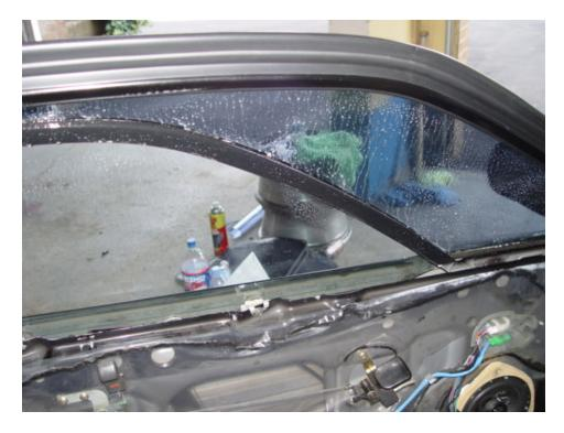
Peel the backing off of the tint and apply it with the sticky side on the glass. There will be some areas where your initial cutting wasn't perfectly accurate. Trim up the edges with a knife.
