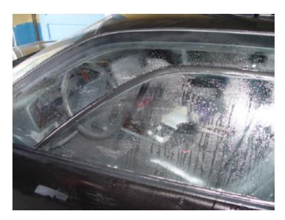
Next, roughly lay a sheet of tint film over the window with the adhesive facing up. The application solution will hold the tint in place so you can begin cutting. This step is to cut the film to the right size.
