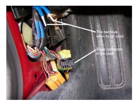
Hold the black connector notch up. With the ignition off, insert one of the wires into the top row,  $2^{nd}$  pin from the left, (see picture below). Turn the key to the on position, **but do not start the car.** Look at the "check engine light" on the dash, and count the blinks. Each long blink = 10 and each short blink = 1. Calculate the number and then check the list of codes to see what the problem is.
