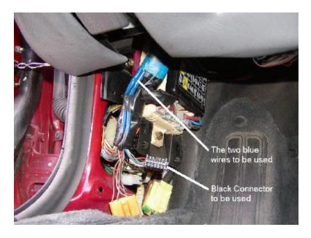
Take the tape off the ends of the blue wires and move them into a position so they can be inserted into the connector.
