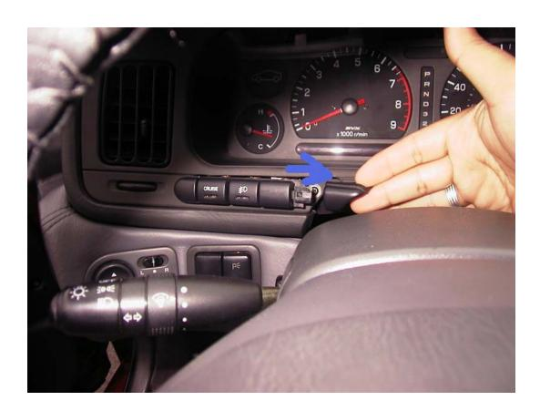
5) Twist the switches around and push them in the hole. Unscrew the 2 screws that hold in the switches, and repeat on the other side.
