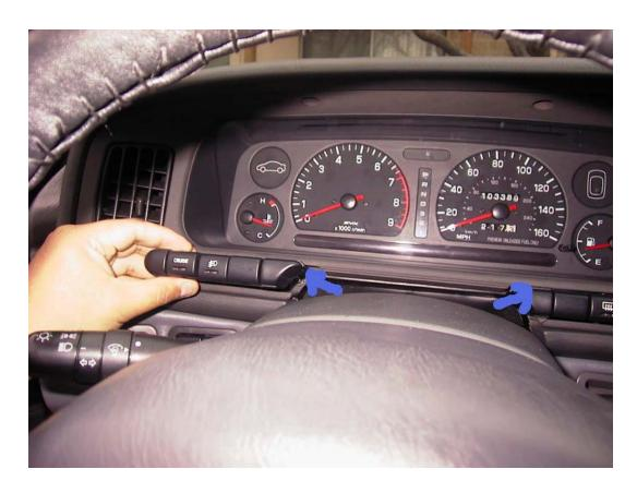
4) Pull off the little tab on both sides of the steering wheel.
