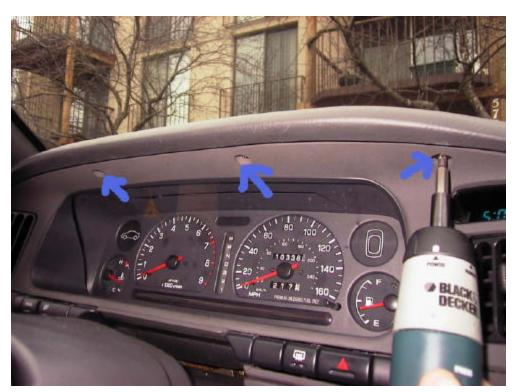
3) Using a screwdriver, pry off these cluster light switches.
