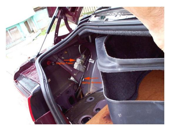
Step 5. Remove two 10 mm nuts and remove antenna assembly from car.
