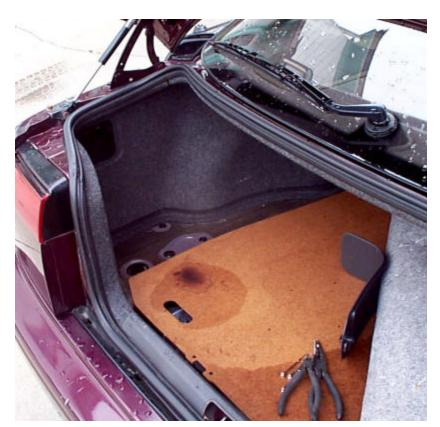
**Step 4.** Peel back trunk liner and disconnect electrical and antenna leads.
