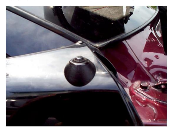
Step 18. Tighten two 10 mm nuts, connect the electrical connector and antenna connector.
