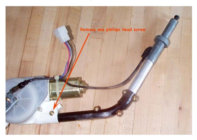
Step 7. Pull mast assembly out until it unwinds all cable and comes loose.
