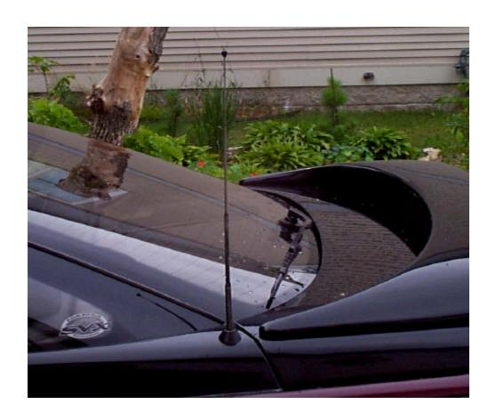
**Step 1.** Unscrew the top using a golf spike wrench or two screwdrivers and a pliers.
