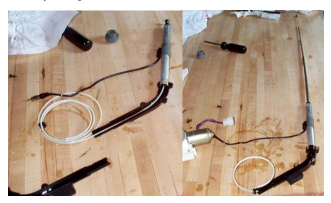
**Step 14.** Slide mast cable into motor a few inches and slide antenna guide and assembly into motor with mast extended. Replace mast screw, zip tie and take back out to car's trunk.
