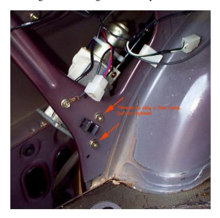
**Step 17.** With your right hand, hold the antenna up through the hole and with your left hand, install the top.
