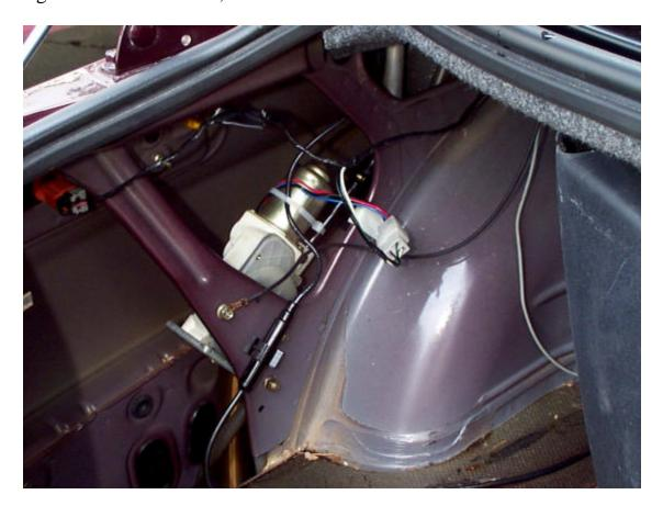
**Step 19.** Connect the drain tube into the rubber grommet so your trunk won't fill with water. Check to make sure the sunroof drain didn't get knocked out of the grommet either.
