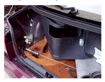
**Step 15.** Lay a rag under the antenna to catch excess oil. Turn on radio for 5 seconds, turn off radio and run and plug in power connector to antenna until it retracts fully. It may take two tries to fully retract. Unplug connector and turn off key.
