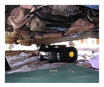
Once that's done, use the 10mm socket on an extension to undo the 20 bolts that hold the transmission pan in place. The pan should drop down very easily, but if not, use a thin pen knife blade to gently pry the pan off. More ATF will drip down once the pan is removed.
