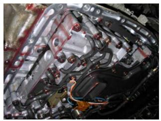
To remove the filter, you'll need to loosen the 4 gold 10mm bolts holding it in place. The filter won't drop out as there's a dark metal tube that runs across one side of the filter. This tube is held in place with 2 black 10mm bolts which will need to be removed as well. The tube can be hard to remove once the bolts are undone, but a gentle tug will soon break it loose.
