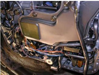
Now, take the new filter and install it, and be sure to use the new rubber o-ring provided that goes around the circular opening that goes up into the transmission.
