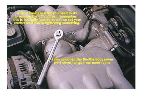
4. Clean the old one or install a new one. It is possible to start threading it by reaching in from the driver's side, towards the back of the engine, under the manifold. It is a tight fit, but easier than trying to start it from the top.
