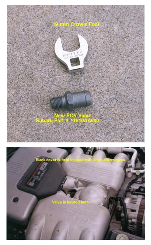
2. Remove the center cover on the intake manifold. It takes a 4mm allen wrench.
