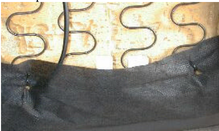
fig 20. Fabric that covers the wiring harness is zip-tied
