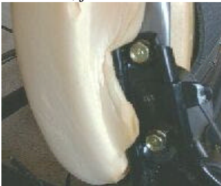
fig 16. Loosen the bolts on either side of the frame to remove the metal rod.
