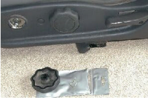
fig 3. Rotary knob removed by prying off metal clip (manual seats only)
