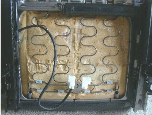
fig 19. Wiring harness clipped back onto the bottom seat cushion
