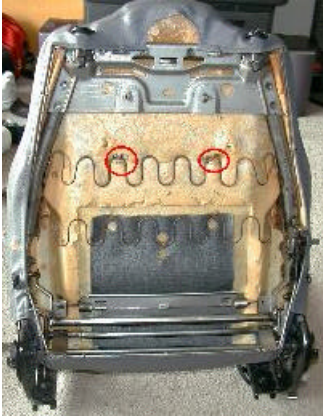
fig 14. Rear of top cushion. Note the additional metal rings that need to be removed.
