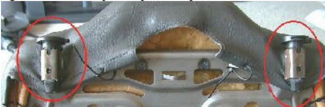
fig 18.3 Top seat cover on under the headrest posts returned to original positions
