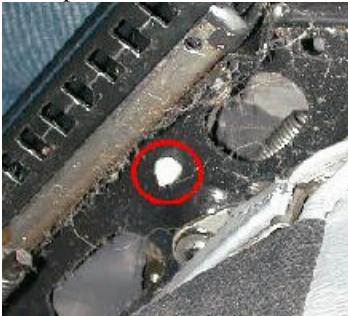
fig 4. Remove the outside plastic cover by pushing on the white plastic push clip
