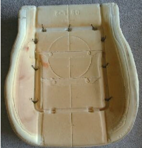
fig 13. Bottom cushion with zip-ties ready for new cover
