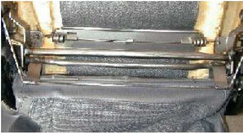
fig 15. Metal rod holding the top seat cover to the frame
