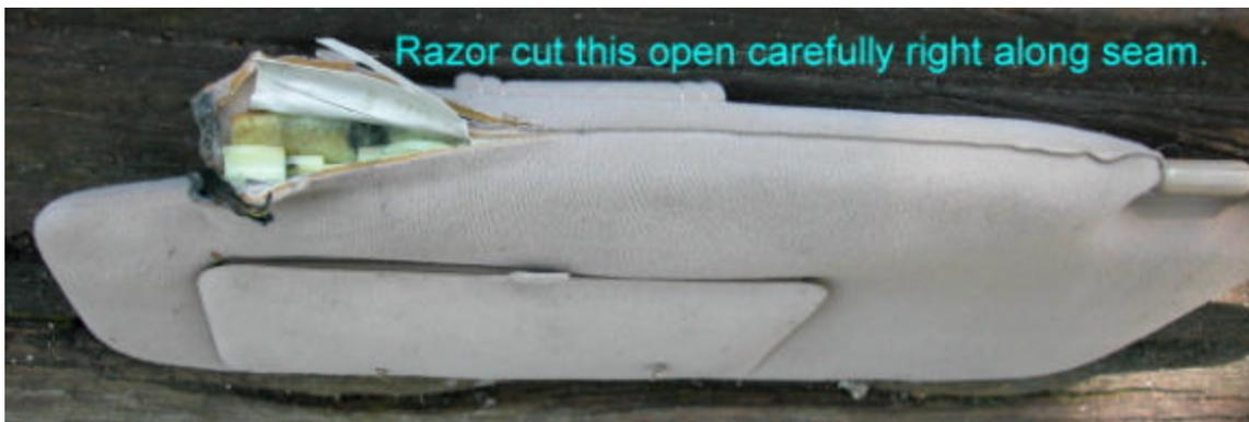
Once you've cut the visor open, you'll find a plastic shaft, that when new, provided just the right resistance for the visor to remain in whatever position you adjusted it to.
