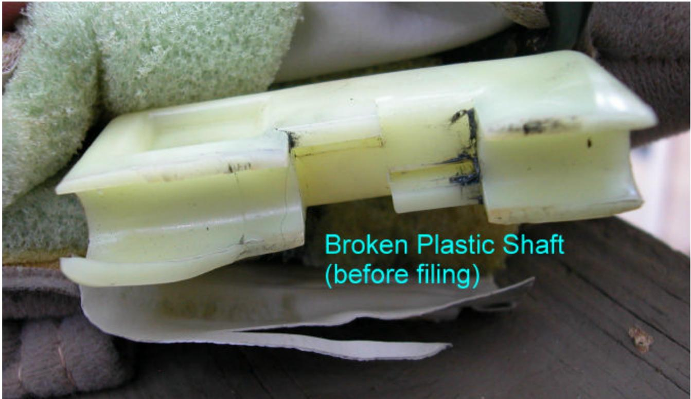
You will find that the notch that is already in the plastic does not have a flat bottom, plus the notch isn't long enough for the Hillman #235 brass insert to fit properly. (To see this once again, GO BACK to the photo before the last two and take a good look at it again)
