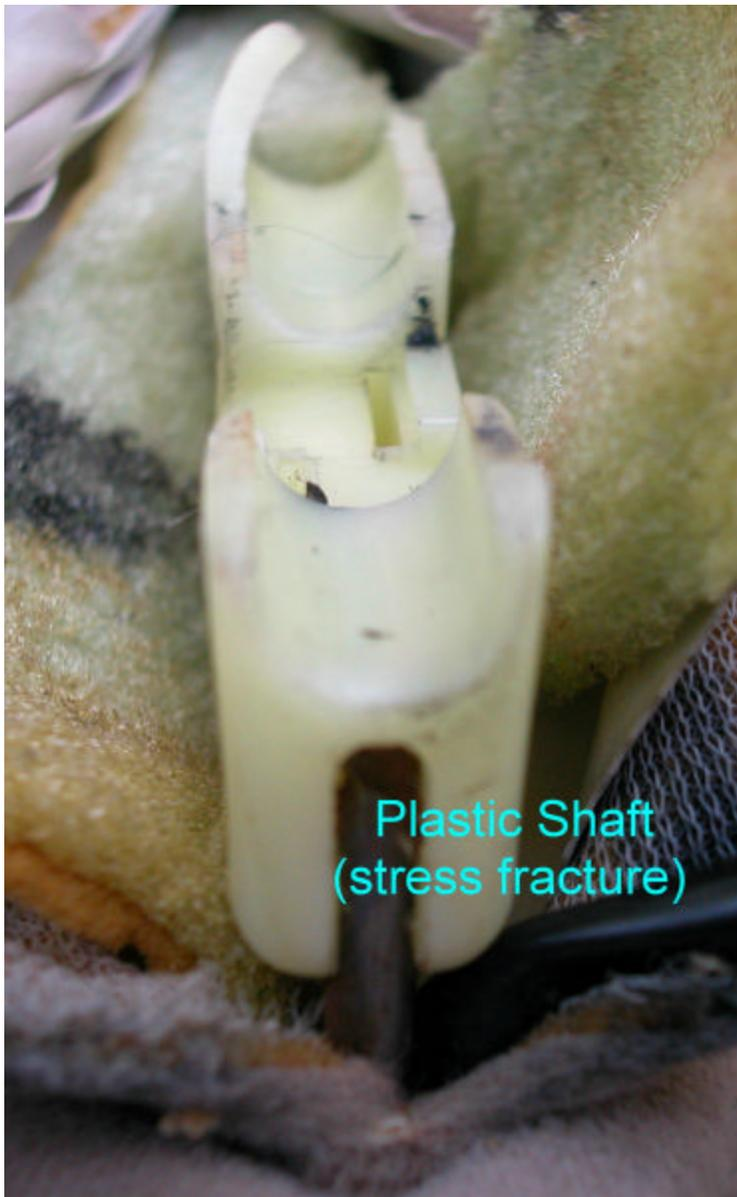
Yours will be different, but I'll bet it may look much the same. The stress and wear and tear on this part causes the plastic to fail, and therefore the visor droops. That's what has to be repaired!
