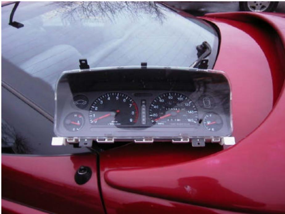
10) Unclip the clips (purple arrows). The green circle is for fuel gauge, blue for temperature, red for the tachometer, and yellow for speedometer. Unscrew them if you want.
