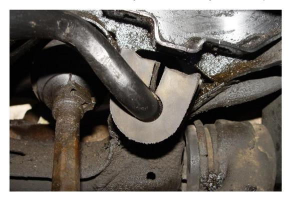
Now slide the retainer bracket over the bushing.
