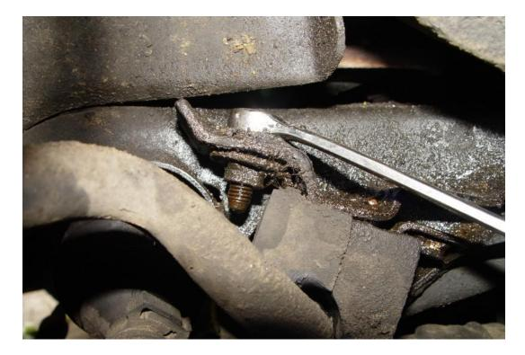
Once the bolts are removed you'll need to pry the retainer bracket straight down with a screw driver or other small tool.
