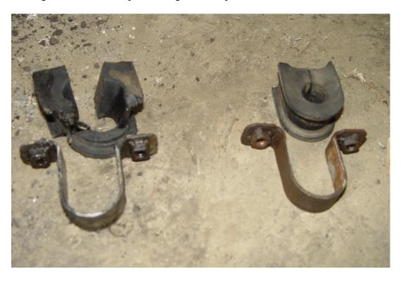
Now it's time to install the new bushing. Place the new bushing around the sway bar.
