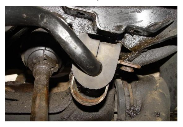
Now, with the bracket fully in place, line up the mounting holes with the flange on the subframe.
