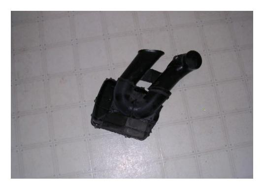
The portion that terminates at the air box doesn't form a seal of any kind with a rubber ring that goes around the opening.
