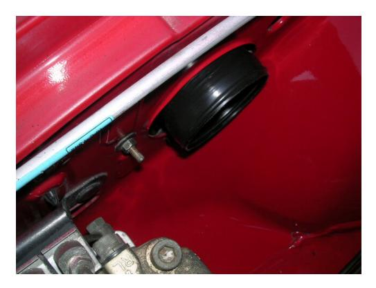
**Step 3:** Test fit the bottom portion of the airbox with the wrapped end of the resonator. Check for a tight, snug, air-tight fit! (if still loose, put more wrap around the resonator until the fit is snug)
