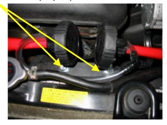
Step 3: Cut bolts provided to about 3/8" long. Be sure to leave the nut ON before the cut to help clear the threads after the cut. Just enough length to go through the bracket and the outter layer of plastic that you just drilled through.
