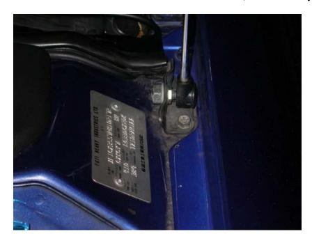
Locate the spot on the hood where the factory lifters would go (you should see a spot on the hood from the mold where the lifters would go) drill a hole the size of the shank of the ball studs.
