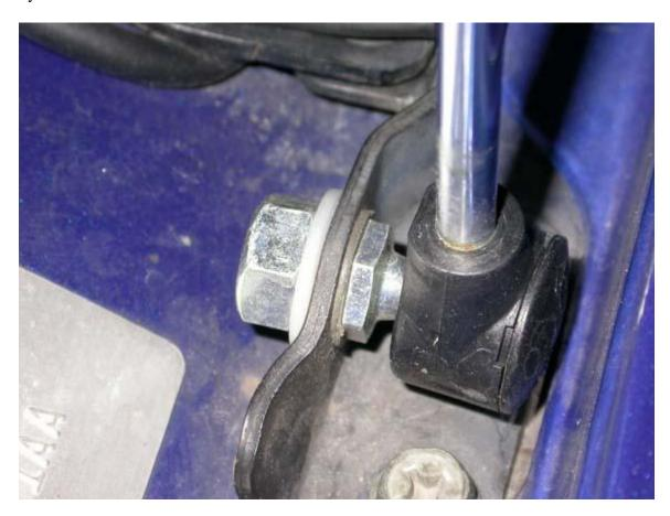
3. Install bracket and ball stud assemble on to car. (Use the factory bolts)
