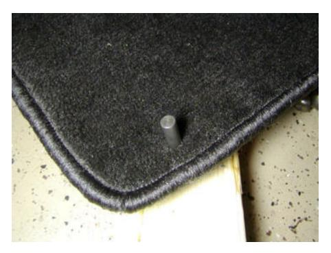
10) Clear out the punched material and insert and set the grommet as per the instructions on the back of the grommet kit. (finished grommet pic below – from underneath). The grommet that comes with the Honda retainer is a nicer black color, but I messed it up on my first try and was forced to use a gold one from the kit. Dayle's mats are so thick that you can't see the gold color when the mat is installed in the car.
