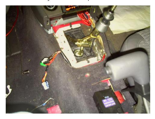
44. Install Custom X-member (may require some grinding to open up bolt holes for proper alignment)
