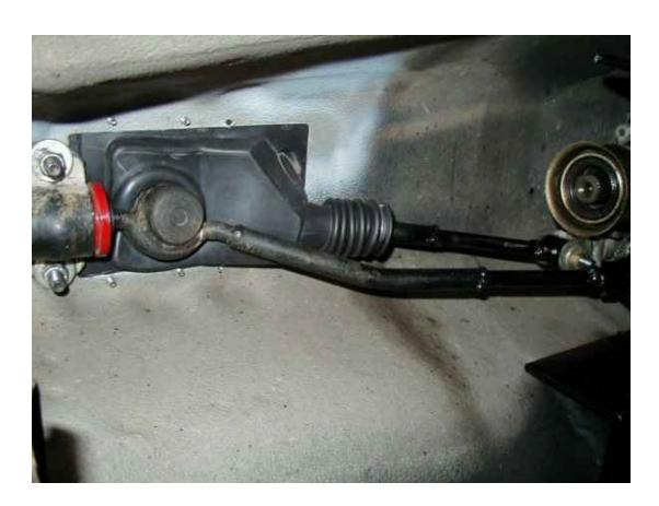
43. Attach rubber boot to body in order to keep road noise to a minimum.
