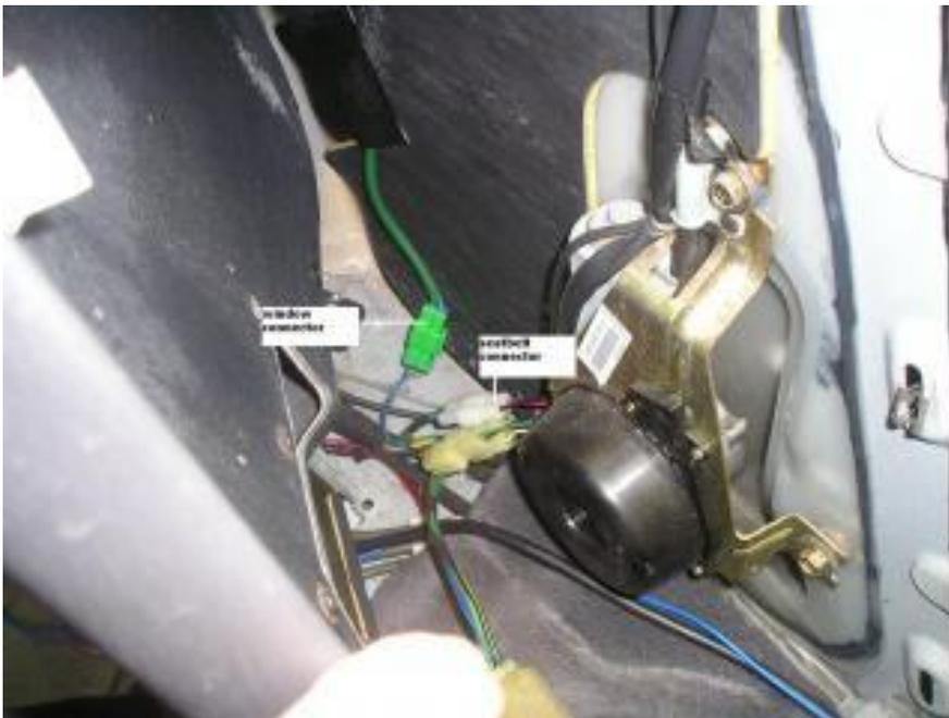
5. Switch the connections (make sure the feed end is connected to the motor). Remember, the connectors are the same type for both the window and the seatbelt motor so you can't make a mistake.
