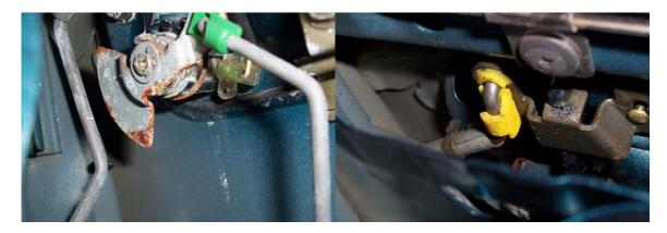
Remove the two 10mm bolts at the 9 and 3 O'clock positions along with the two screw at the 5 and 7 O'clock positions.
