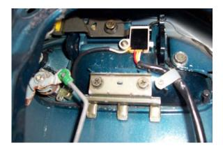
The door handle can be removed now. Be careful not to damage the wires.
