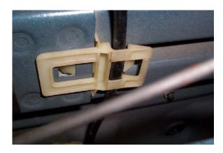
Release the green (lock) and yellow (latch) rod clips from the handle.
