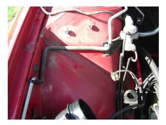
4) Unbolt the engine oil filler tube.
