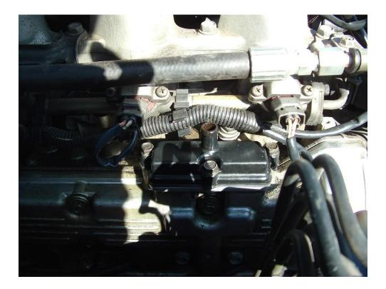
6) Here are a couple of pictures of where the bolts are. Remove the ten bolts that hold each valve cover on.
