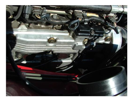
11) Replace the coils with the bolts that were removed before. (3 on each side)
