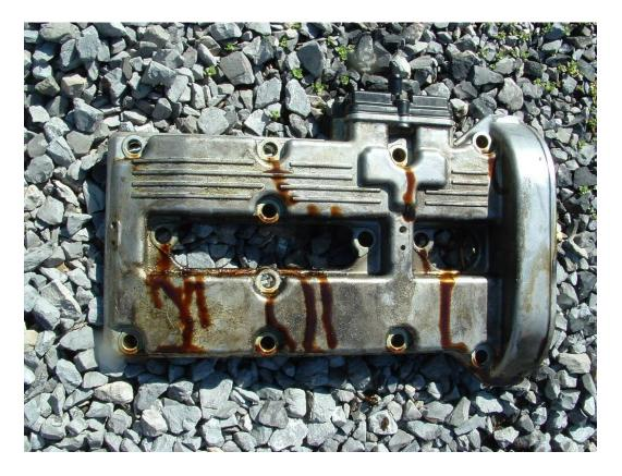
7) Take the actual valve cover over to a bench and remove the three rubber seals. They're relatively easily to remove (one goes all around and the other two go around the middle area where the coil packs sit).
