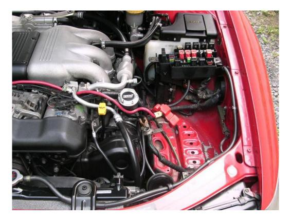
2) Unscrew the 2 clamps from the intake that goes onto the throttle body and MAF.
