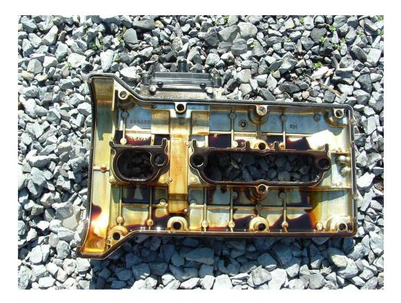
8) Replace the seals with the new ones. Note that the seals are specific to one side of the engine. When putting in the new gaskets remember to clean the groove and edges on the motor and the covers so everything will seal properly. Don't force the new seals down into the little grooves, but push them in gently (if the rubber is damaged during installation, the seal will fail)
