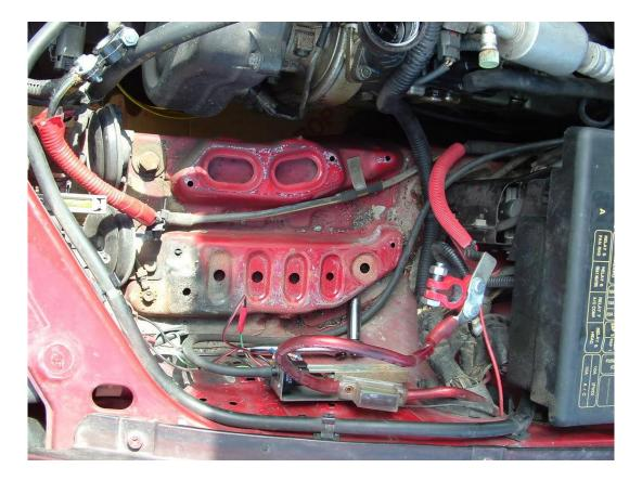
Here's a picture of the valve cover. The black wire in the middle of the picture can be moved to the left so it's not in your way.
