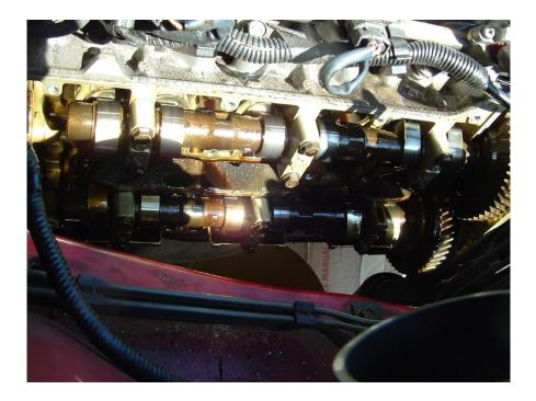
9). Remember to replace the old washers with the new ones. There are two bolts that are smaller than the rest. They go into the holes closest to the firewall.
