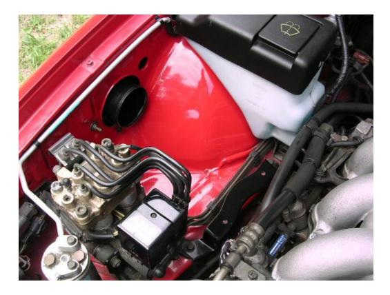
3) Remove the top of the washer fluid container and remove the 2 screw/bolts and pull it up, but remember to unplug the pump and take the rubber hose off at the bottom.
