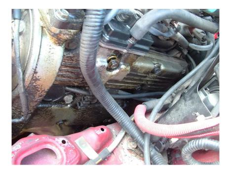
13) Remove the coils, tubes and wires needed to get the valve cover off like you did on the first side.
