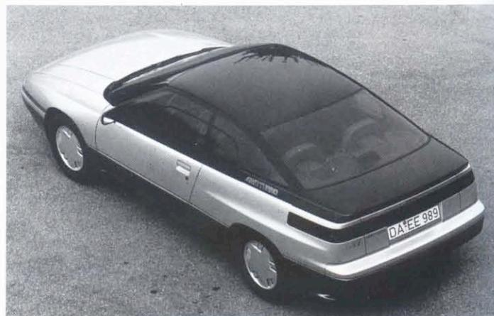
*SVX has soft and curved lines, but does not give in to the temptation of the latest, somewhat bland, 'all round' fashion. A flank of wedged profile contributes, together with the canopy, to a Cd of 0.29. Vertical bulk of the bonnet was limited thanks to the adoption of polyelliptical headlights and a six cylinder boxer engine.*
