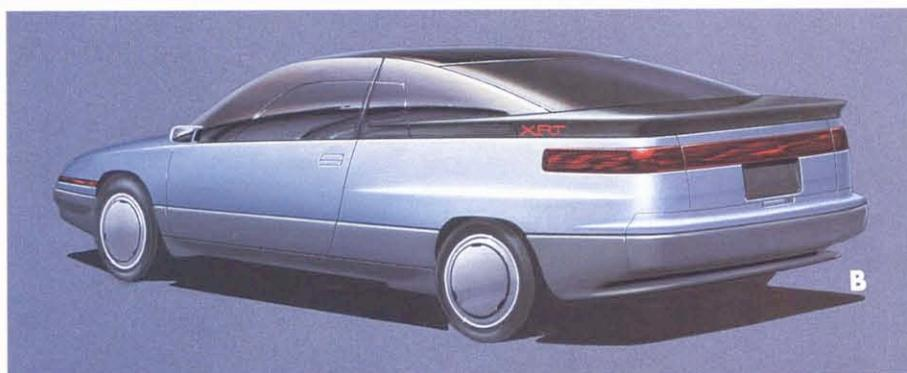
From the top, formal research in the definitive phase. The car underwent few modifications with respect to the Italdesign project illustrated here, including the substitution of concealed headlights for a normal setup of limited height.
