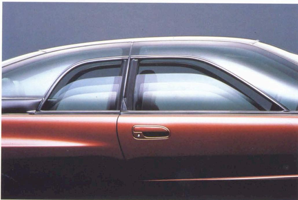
Detail of lateral glasswork evidences the fixed glazed arc, joining up with the fibreglass top to form a dome. Above, the SVX in front and rear views. Design of the grille comes from the Subaru style centre.
