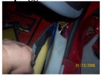
Next thing is to run the wire in the car to the trunk. I ran the wire along the side board of the passenger seat to the trunk. See Pictures above. Must remove the plastic part, underneath the door. It pops off and will pop right back in. Run the wire all the way to the empty back seat. Fold the seat down and run the wire to the trunk by using the side. You will see it, as I don't have a picture of putting it through there.
