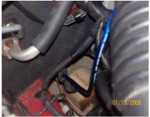
This is an image of the wire running through the hole. I was able (once running the wire) to put the drain hose back on and through. After running the wire you will need to get it over to the batter terminal by running the wire behind the intake and behind the brake cylinder.
