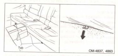
(2) Insert the hexagonal wrench (provided on the bottom surface of the center console) into the side panel hole and slowly turn the wrench clockwise until the shoulder belt anchor locks at the rear end.
