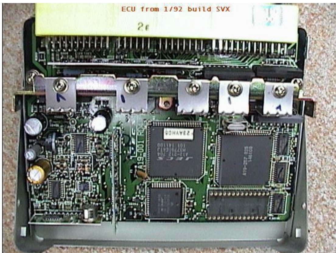
1/92 ECU – With Resistor and Black Noise Suppressor Bead
