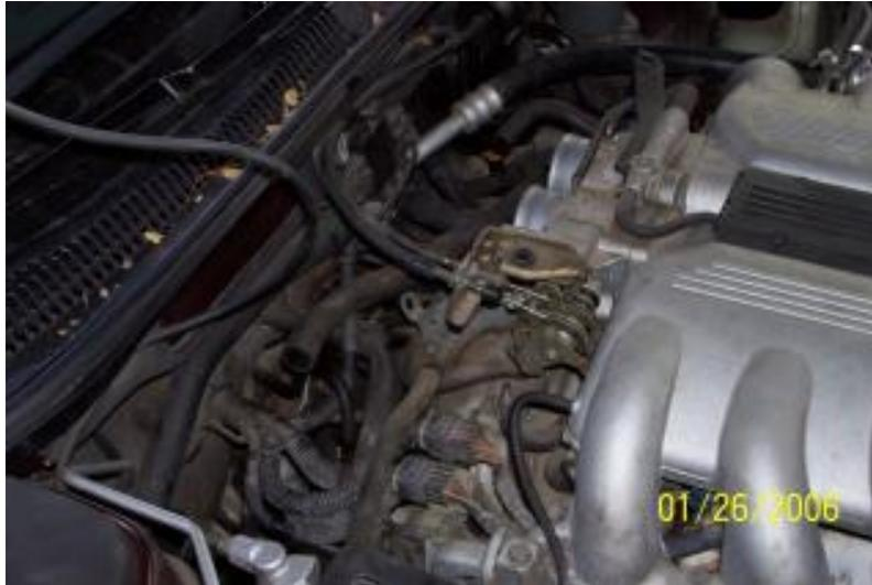
4. Now, you are ready to begin. The hose clamps are  $\frac{1}{4}$  inch sockets with a flathead slot. You will be much better using the  $\frac{1}{4}$  socket than a screwdriver, as the room to work with is extremely cramped. Look closely in the following picture, at the center of the picture on the left side. You can see the screw shining right below the closer electrical connection.
