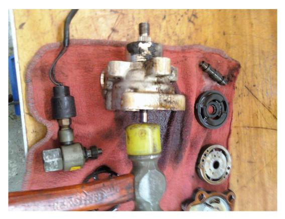
10. Take note of the shim/washer that comes out when the shaft is separated.
