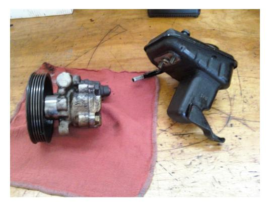
3. Remove the four 14 mm bolts from the back of the pump, throw the old gasket away. NOTE THE POSITION OF THE GUIDING PINS!
