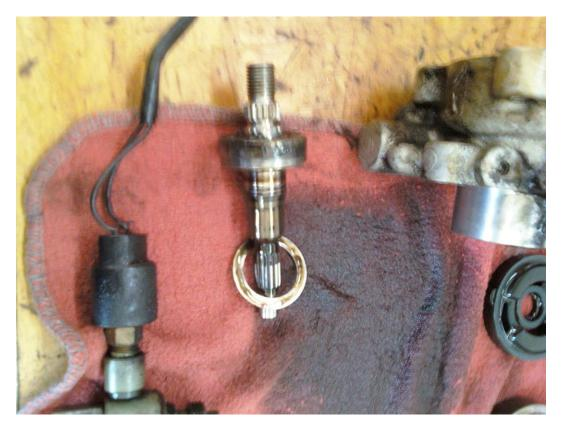
11. Remove the Shaft seal using a punch or pick. It's kind of tricky because you don't have much room to get it. Knock it out from the back side.
