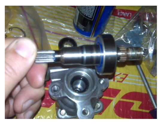
15. Set the front housing on a vice (with a rag or something under it to keep it from messing up the mating face) and hammer the shaft back into the housing using the 24mm socket.
