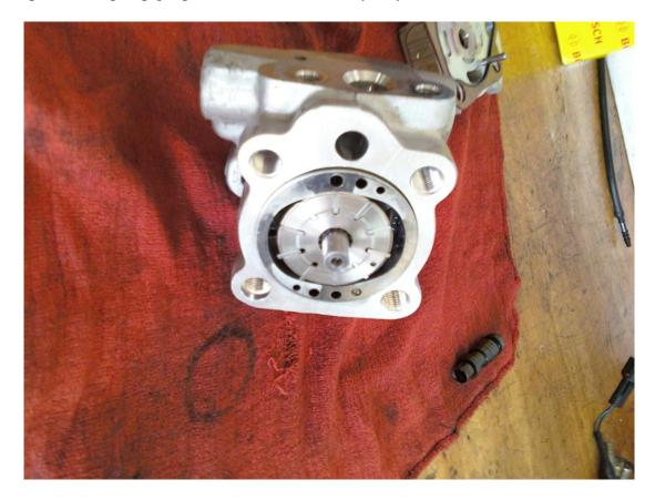
19. Install the new gasket, NOTE THE GUIDING PINS, reinstall the back cover. Tighten the four 14 mm bolts in torque sequence, like a star pattern for a wheel. At first it looks like the pump won't go back together, but the bolts will eventually compress the new O-rings.
