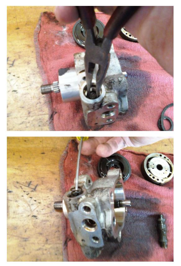
8. Use the snap ring pliers to remove the spring loaded c-clip holding the shaft into the housing.
