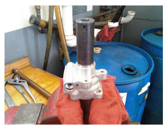
16. After the shaft has been driven all the way down, you will be able to see where the snap ring rests. Reinstall the snap ring.
