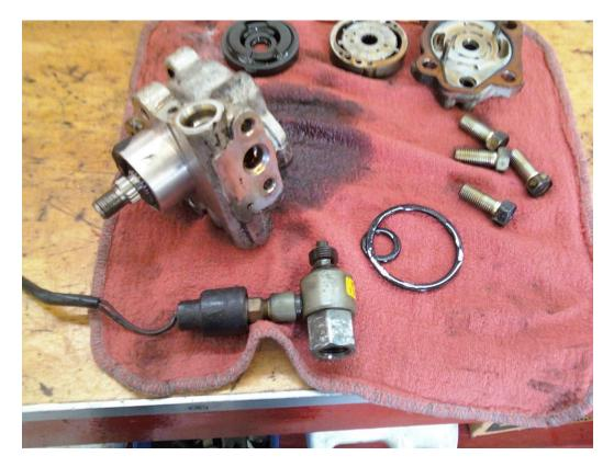
7. There is a spring behind the piston in the output portion of the pump. Replace the spring because its good practice and any spring will eventually loose tension. Again: NOTE THE DIRECTION OF HOW IT COMES APART. LAY IT OUT IN THE ORDER IT WAS REMOVED.
