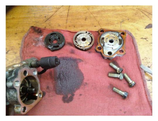
5. Remove the 2 - O-rings in the front portion of the case.
