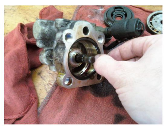
6. Carefully put the pump in the vise being careful not to scratch any mating surfaces, and loosen the 22 mm high pressure output flange.
