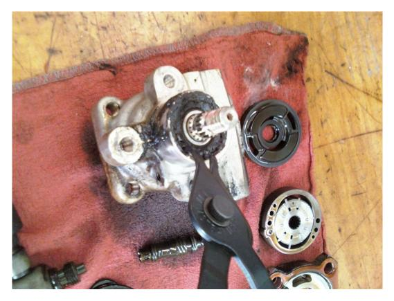
9. Use a soft hammer or a block of wood to bang the shaft out of the housing. Hit the shaft from the back towards the front of the pump.
