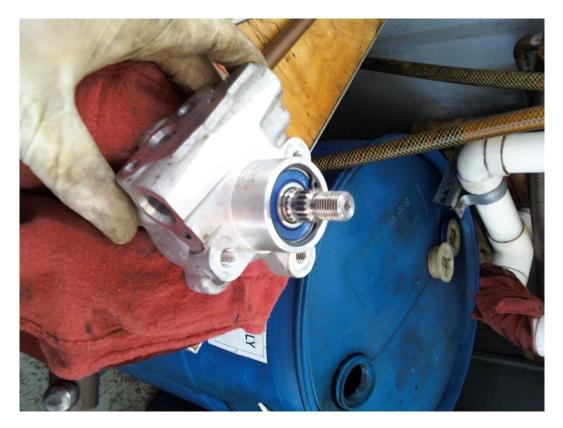
17. Flip the pump over and install the 2 new O-rings.
