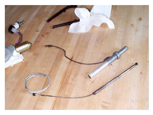
**Step 10.** If you are replacing your antenna mast, skip to step 11, otherwise, clean your mast and cable until all the grease is off.
