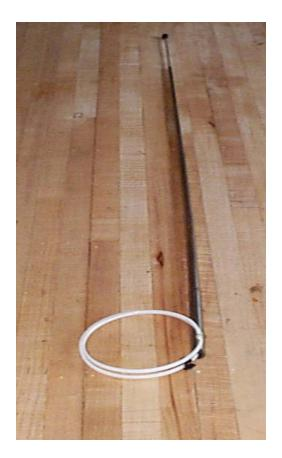
**Step 11.** Oil your cleaned or new mast with a lightweight oil. I used Air Tool oil. Extend and retract while spreading oil all over with a rag or fingers until mast and cable are well oiled.
