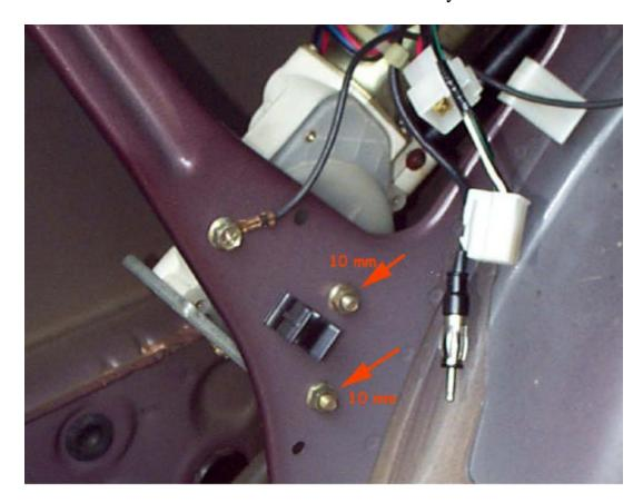
Step 6. Remove mast screw and slide off zip tie.
