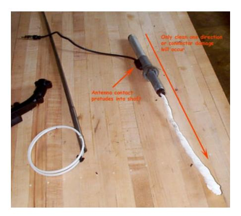
**Step 13.** Slide the oiled mast into the oiled shaft. Fit mast/shaft assembly into bottom half of guide. Place top half of guide on and re-install the four screws.
