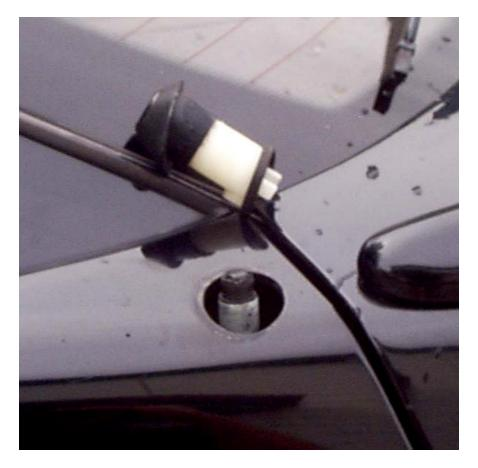
Step 3. Peel back carpet and remove left taillight bulb access panel.
