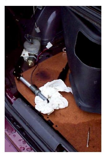
**Step 16.** Slide antenna assembly up through the hole and install the two 10 mm nuts just enough to keep it from falling off. Do not tighten the nuts yet.
