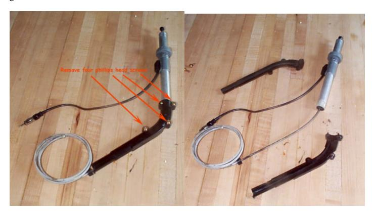
Step 9. Slide antenna mast out bottom of shaft.
