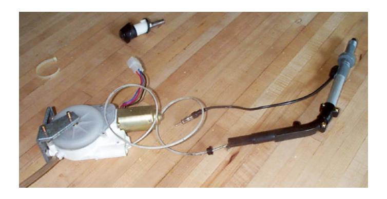
**Step 8.** Remove four screws holding the mast guide. Separate the top and bottom half of mast guide.
