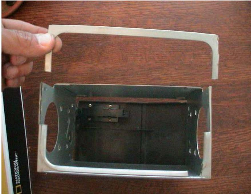
You will have to modify the bracket (above). You don't have to cut all the edge off, only enough to get the unit in. You will need to notch for antenna. (bottom right)
