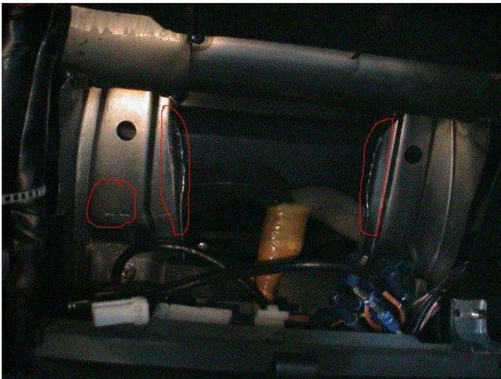
These were bent out of the way instead of being cut. The two flanges (highlighted with long circles) may need to be cut or bent back out of the way.
