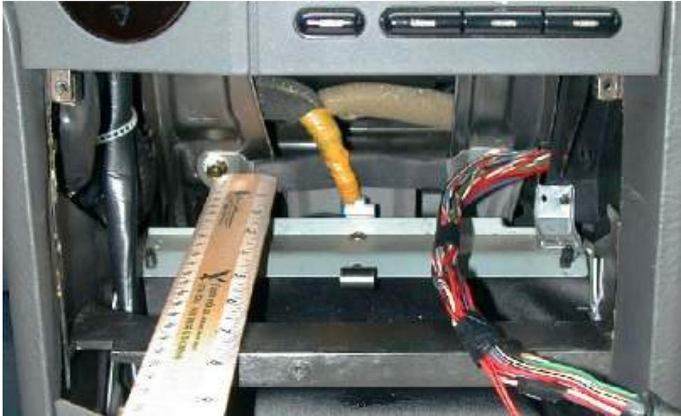
On the inside edge of the two struts is a flange that points towards the rear of the radio. These are what touch the rear of the WRX radio and keep it  $\frac{1}{4}$ " out. The upper halves of these flanges need to be cut out or bent out of the way.
