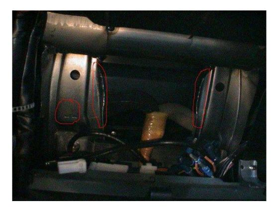
These were bent out of the way instead of being cut. The two flanges (highlighted with long circles) may need to be cut or bent back out of the way.
