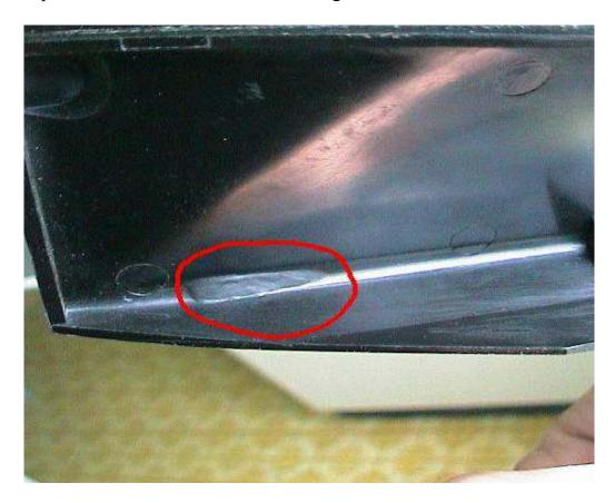
When grinding, be careful not to grind all the way through the cover. You will start to notice where it is getting thin or starting to blister on the back side when you are almost through the cover. (see red circle)
