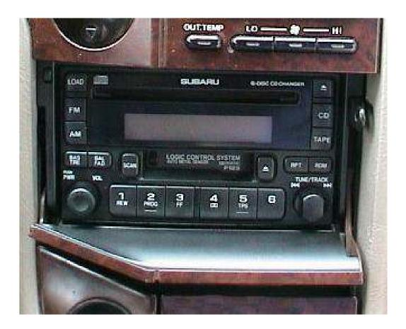
Here is the finished product. The slight grinding allows the door to go up like it is a stock unit. Be sure to mount the trim piece around the sides of the unit.
