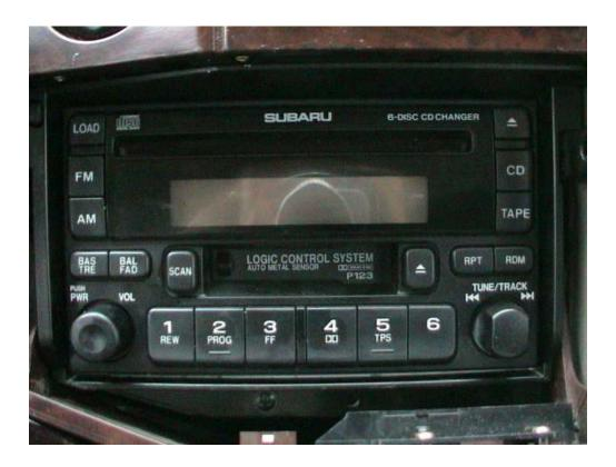
The unit is now installed. The antenna wire needs to be plugged in before sliding in the unit. Use one of the two – the one with the male plug. Most radios will require an 18" or 24" antenna extension cable to reach the SVX's antenna cable.
