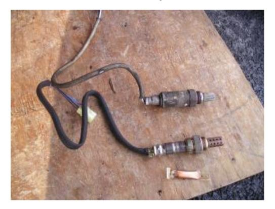
7. Apply lube to the threads of the new sensors before installing.
