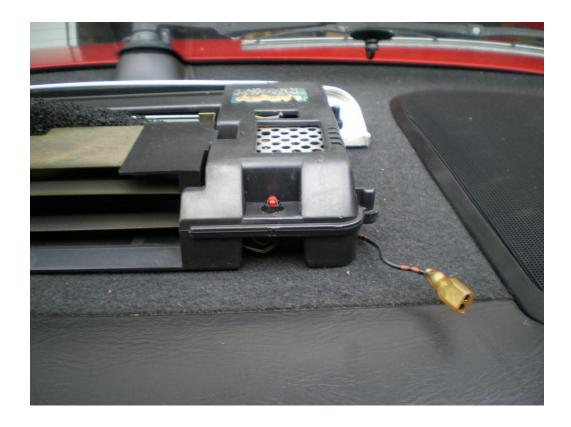
The high voltage ionizer plates are removed (along with the charcoal filter) which shows the blower fan.
