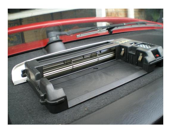
The high voltage plates & charcoal filter are out of the unit.
