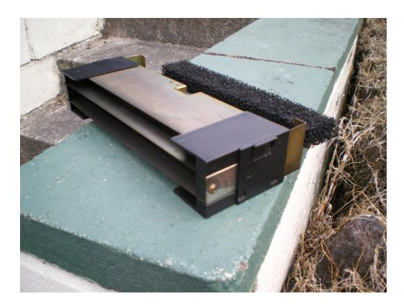
The outside plates are joined to form a shield. The inner plates are also joined and these are the High Voltage ones!!
