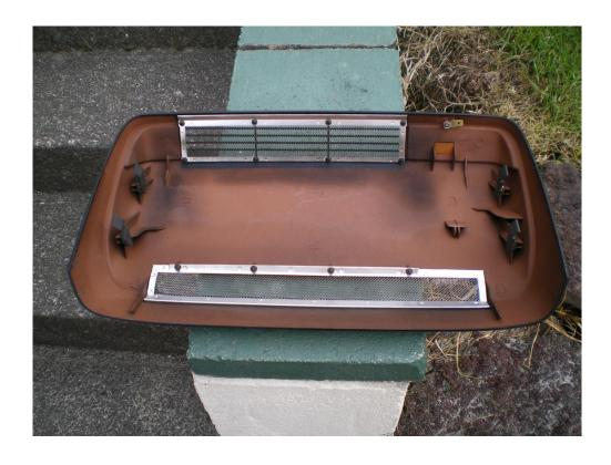
The metal plates are the high voltage parts (2Kv +). Replace lamp with LED, and notice the micro switch that fits in with the previous photo. Disable high volatge when the cover is off. The charcoal filter is just behind the plates & a fan is behind that.
