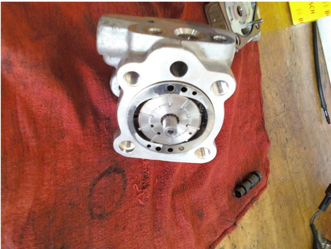
19. Install the new gasket, NOTE THE GUIDING PINS, reinstall the back cover. Tighten the four 14 mm bolts in torque sequence, like a star pattern for a wheel. At first it looks like the pump won't go back together, but the bolts will eventually compress the new O-rings.
