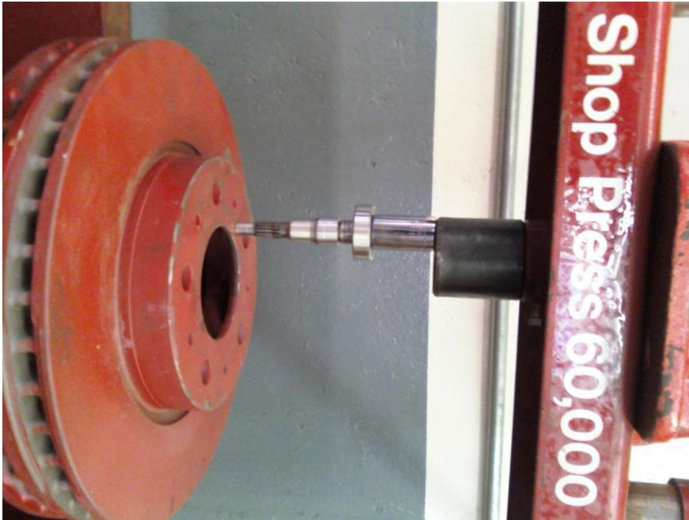
14. After you clean everything off, you can begin the reassembly process. Press the new shaft seal into the front housing using the 20mm socket. Put the shim/washer on top of the seal.
