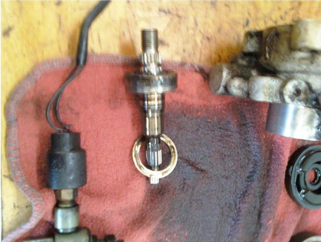
11. Remove the Shaft seal using a punch or pick. It's kind of tricky because you don't have much room to get it. Knock it out from the back side.
