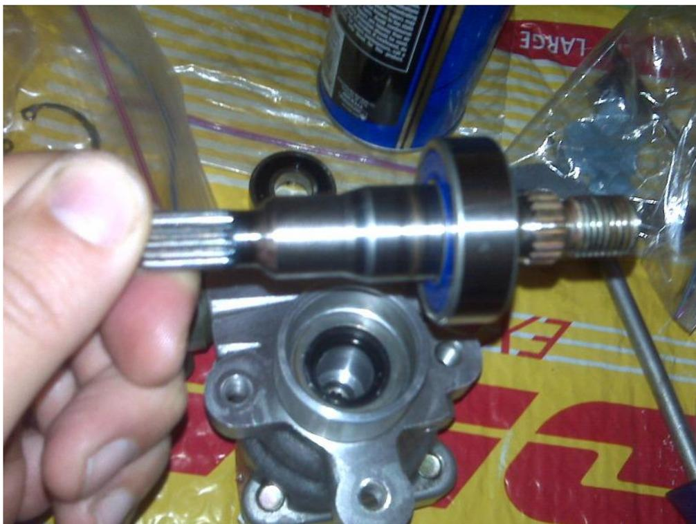
15. Set the front housing on a vice (with a rag or something under it to keep it from messing up the mating face) and hammer the shaft back into the housing using the 24mm socket.
