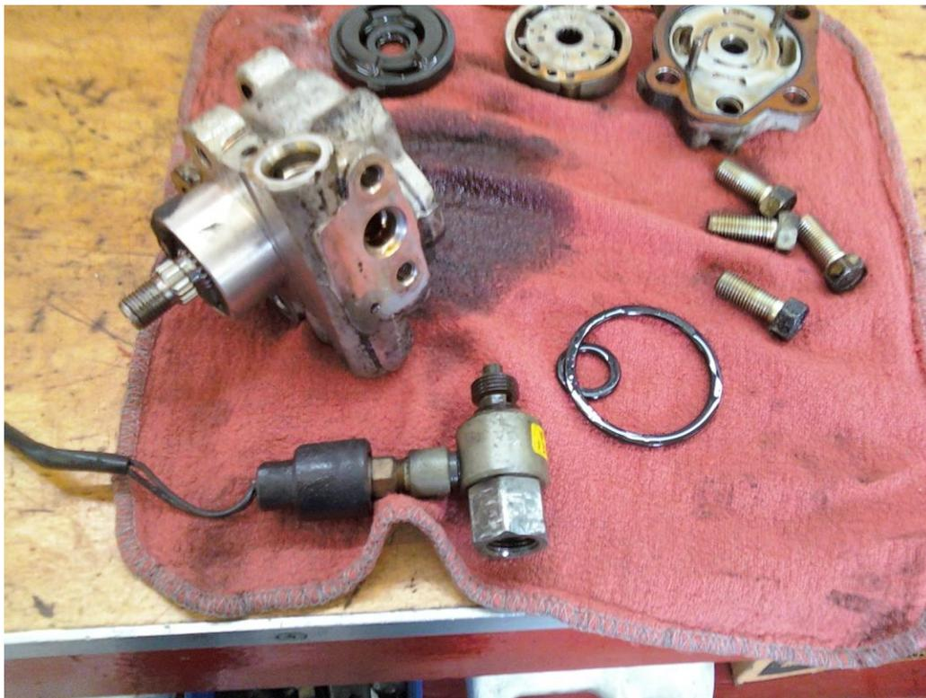
7. There is a spring behind the piston in the output portion of the pump. Replace the spring because its good practice and any spring will eventually loose tension.
