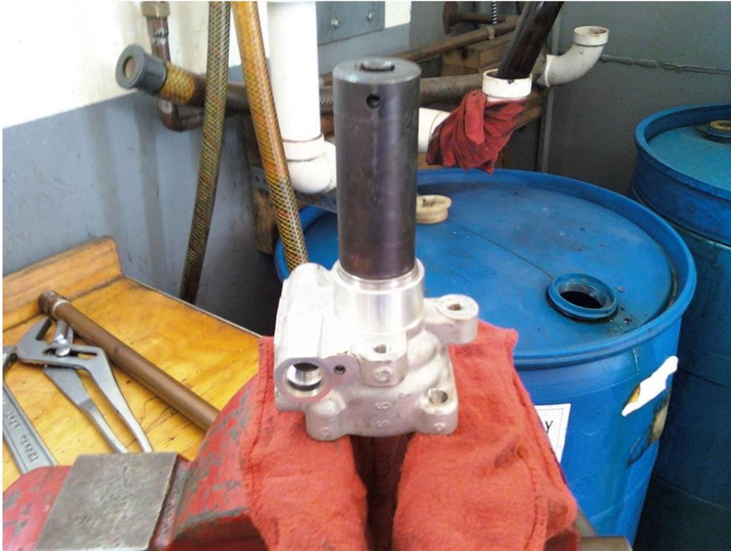
16. After the shaft has been driven all the way down, you will be able to see where the snap ring rests. Reinstall the snap ring.
