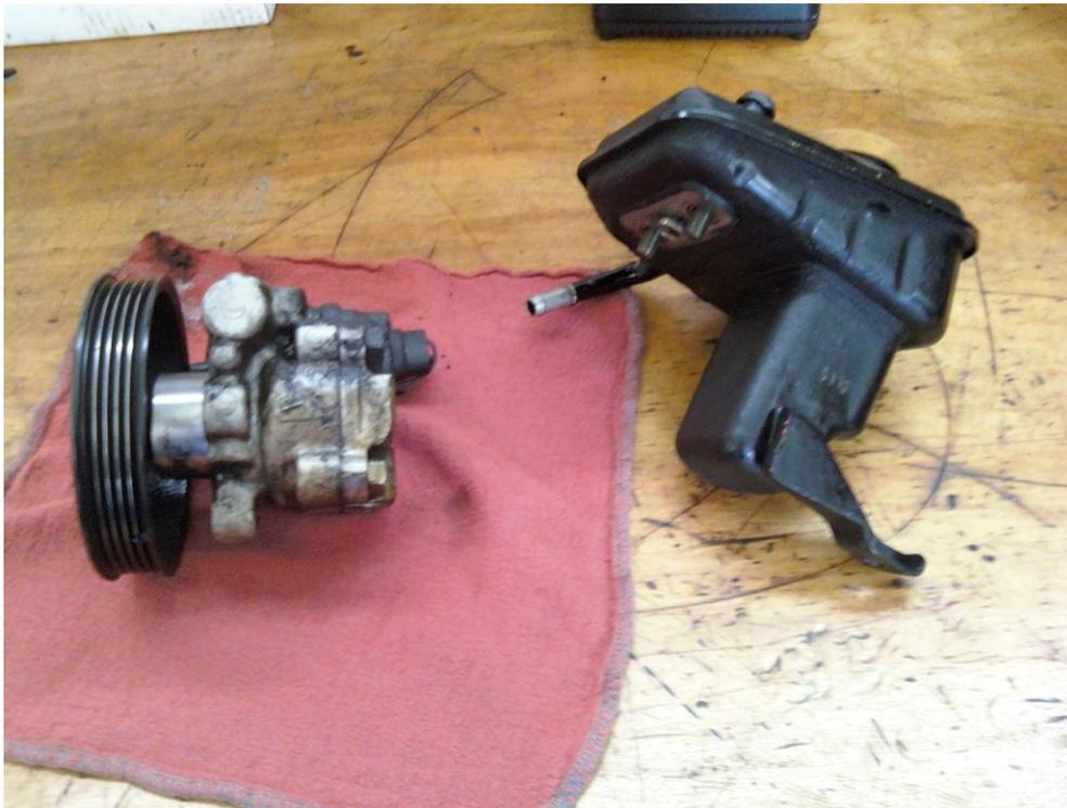
3. Remove the four 14 mm bolts from the back of the pump, throw the old gasket away.
