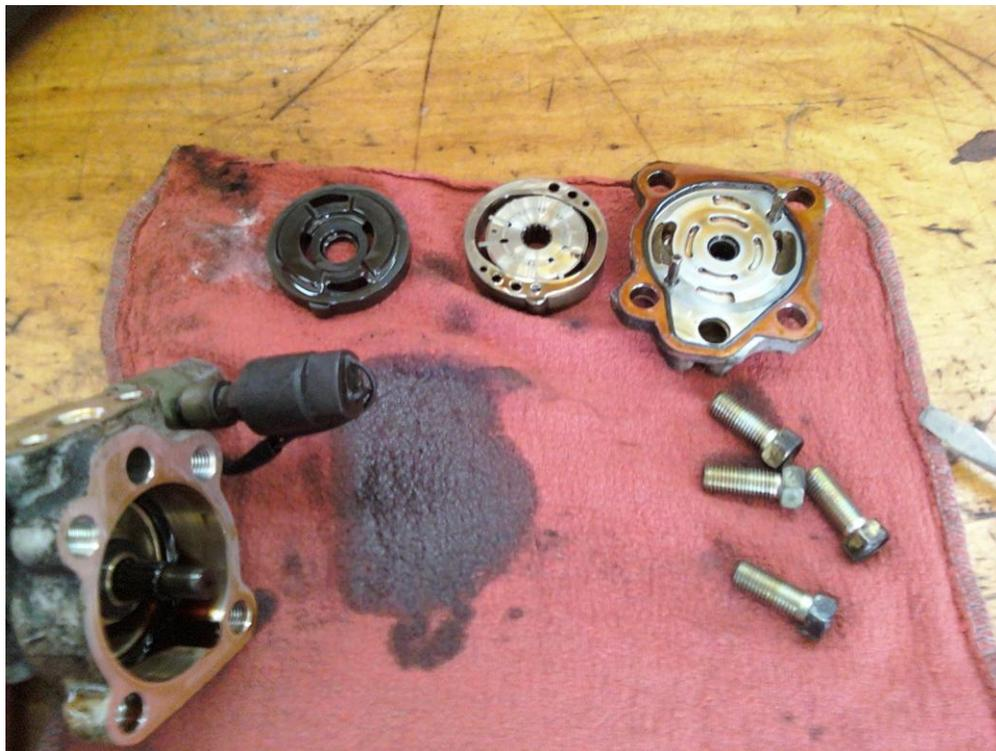
5. Remove the 2 - O-rings in the front portion of the case.
