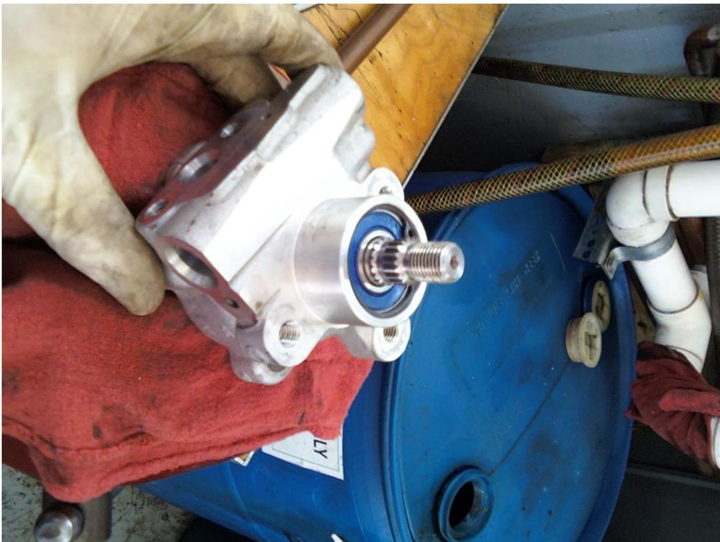
17. Flip the pump over and install the 2 new O-rings.
