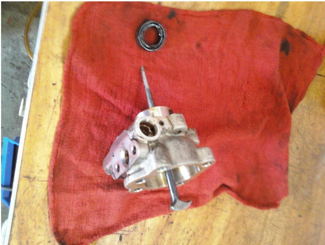
12. Take the shaft over to the press and use the 20mm socket to press the bearing off the shaft. It will go towards the front of the shaft.
