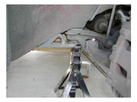
3. Remove the 14mm bolt and nut. Then push down on the A-arm to break loose the ball joint shaft from the wheel hub. You don't have to slide it out all the way yet. Remove the three 17mm bolts and nuts. Push down on the A-arm while trying to slide the ball joint out. It takes a little bit to get it out, so keep working at it.
