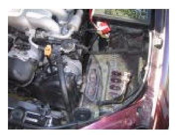
You will notice that the plug wires are different than other cars. Each plug has its own coil for power instead of using a master coil that provides power to all of the plugs. You can see in the picture below, two of the coils. There are 12 mm bolts that hold each individual coil in place. You can start with the one on the right, closest to the front which is very easy to get to. This will allow you to see how to change one before you get to the hard ones.
