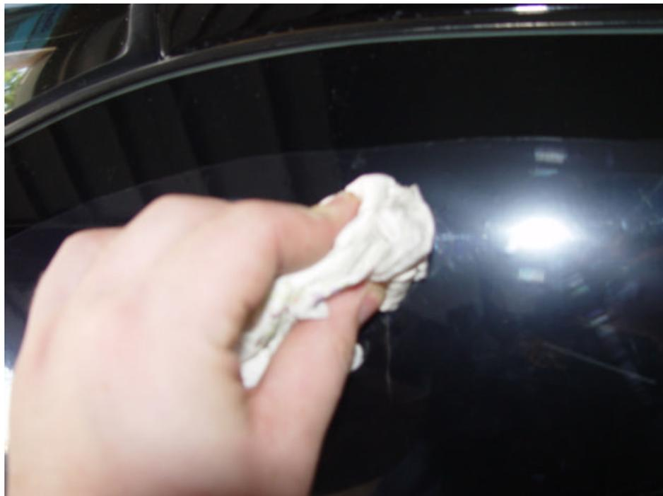
Remove the inside door panel and soak the inside of the window. Make sure the window is clean and free of any dust or decals.
