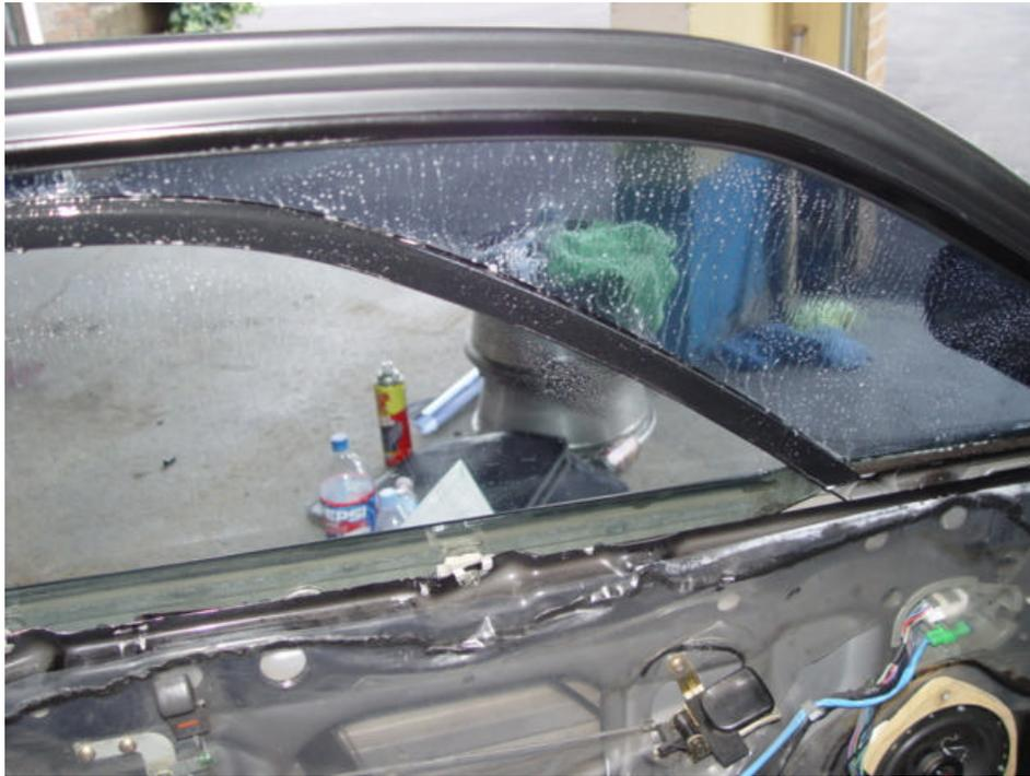
Peel the backing off of the tint and apply it with the sticky side on the glass. There will be some areas where your initial cutting wasn't perfectly accurate. Trim up the edges with a knife.
