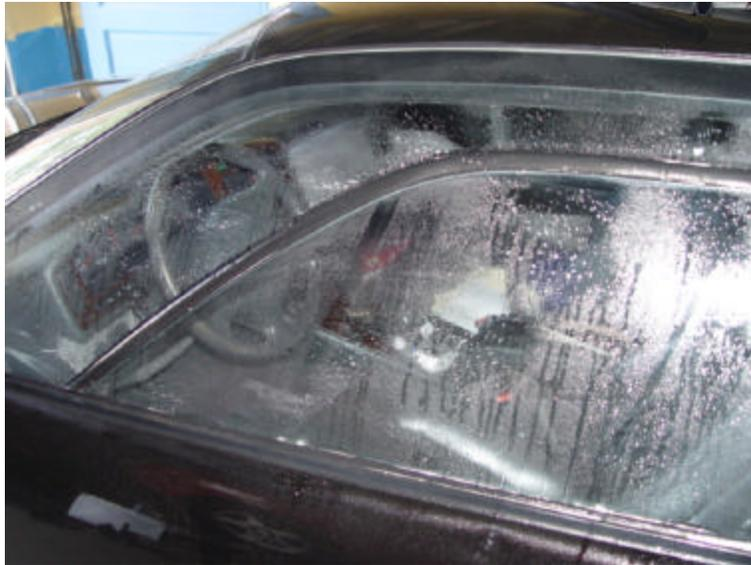
Next, roughly lay a sheet of tint film over the window with the adhesive facing up. The application solution will hold the tint in place so you can begin cutting. This step is to cut the film to the right size.
