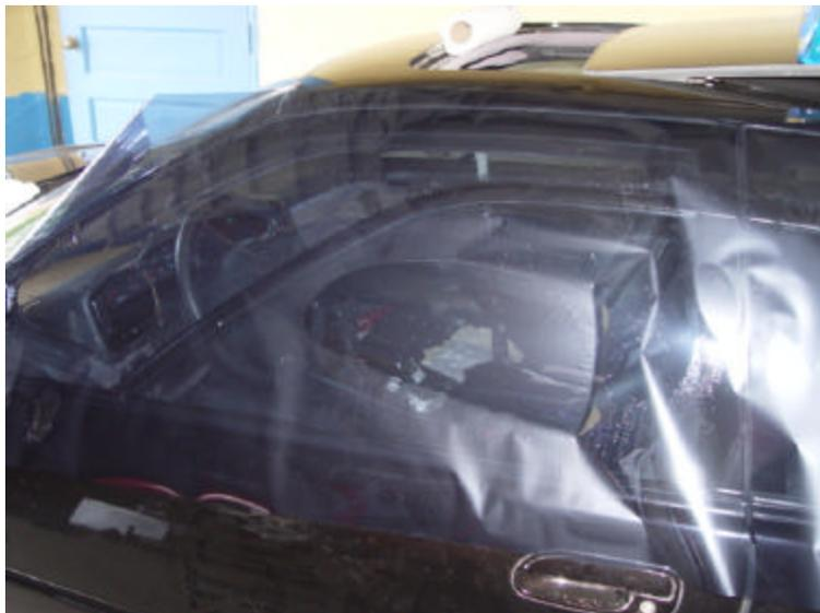
Cut the film so that it lines up with the inside edge of the glass (the clear part). It's OK to leave some additional tint at the bottom, since this part will go below the door panel on the inside of the window.
