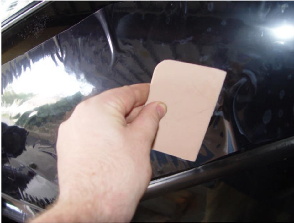
These lines will not smooth out just by using the bondo knife. You'll need to heat them up. Apply some heat to them, one at a time, with the heat gun, and smooth them out with a bunched up paper towel. This is the most difficult part of the process, so take your time. It takes a while to figure out exactly how much heat to apply. This is still on the outside of the window to get the proper shape. The tint will be applied to the inside in the next couple of steps.
