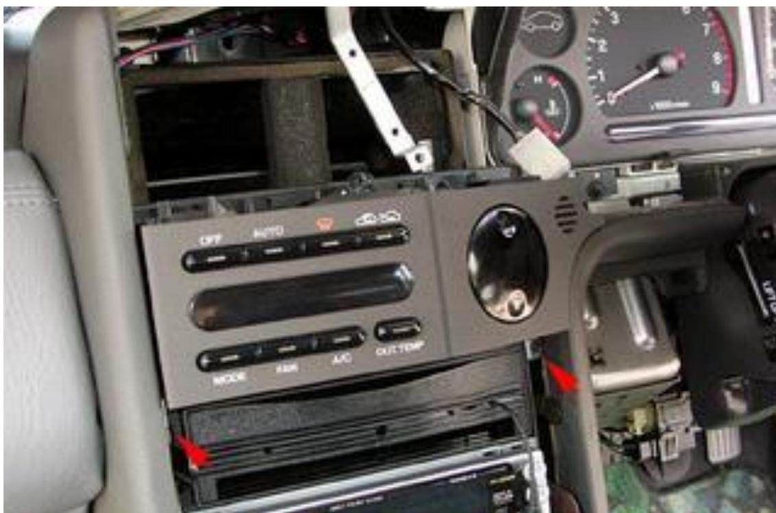
Pull unit out at an angle: all the wiring harness connectors are towards steering wheel side so pull and swivel towards steering wheel.
