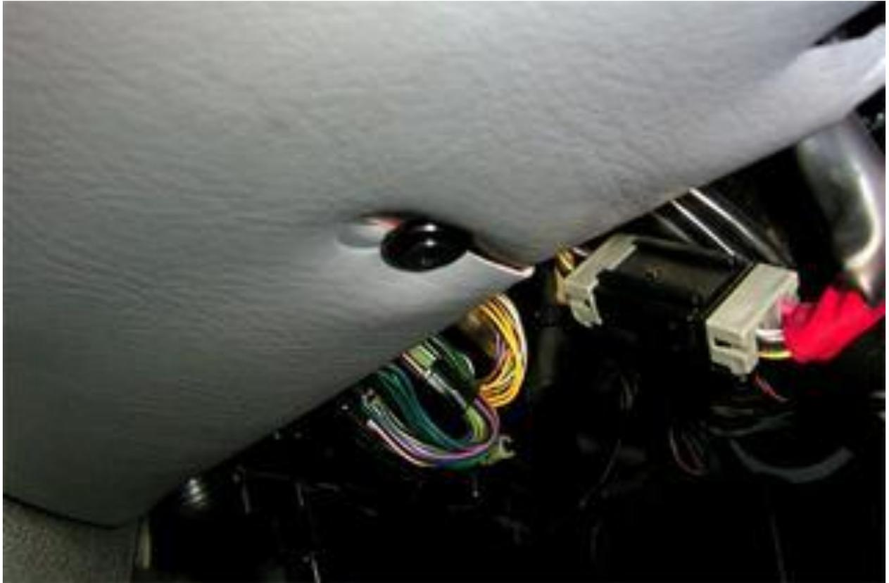
Once removed, the cover is held on by only 2 spring clips that are halfway down each side (see the “prongs” in photo 2 below) pull & it will come away, BUT there are still 2 electrical connectors that need to be unmated (see the below): -
