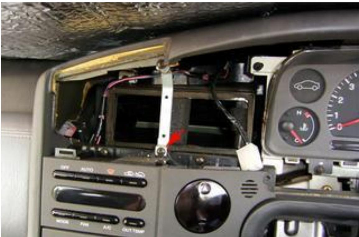
Remove the 2 screws on top as indicated.
