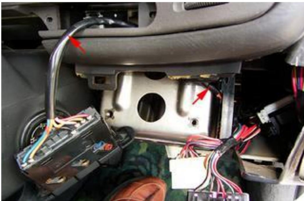
Remove the 3 upper screws from under the instrument cluster.
