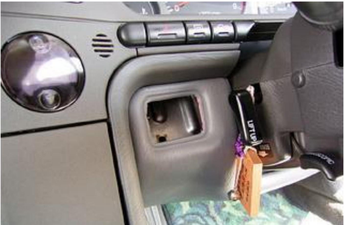
Pull forward both sets of switches (Park and Mirrors) and remove them from joining connectors (if you cannot do it at this stage then leave till later on – it is easier to do as you remove more pieces).
