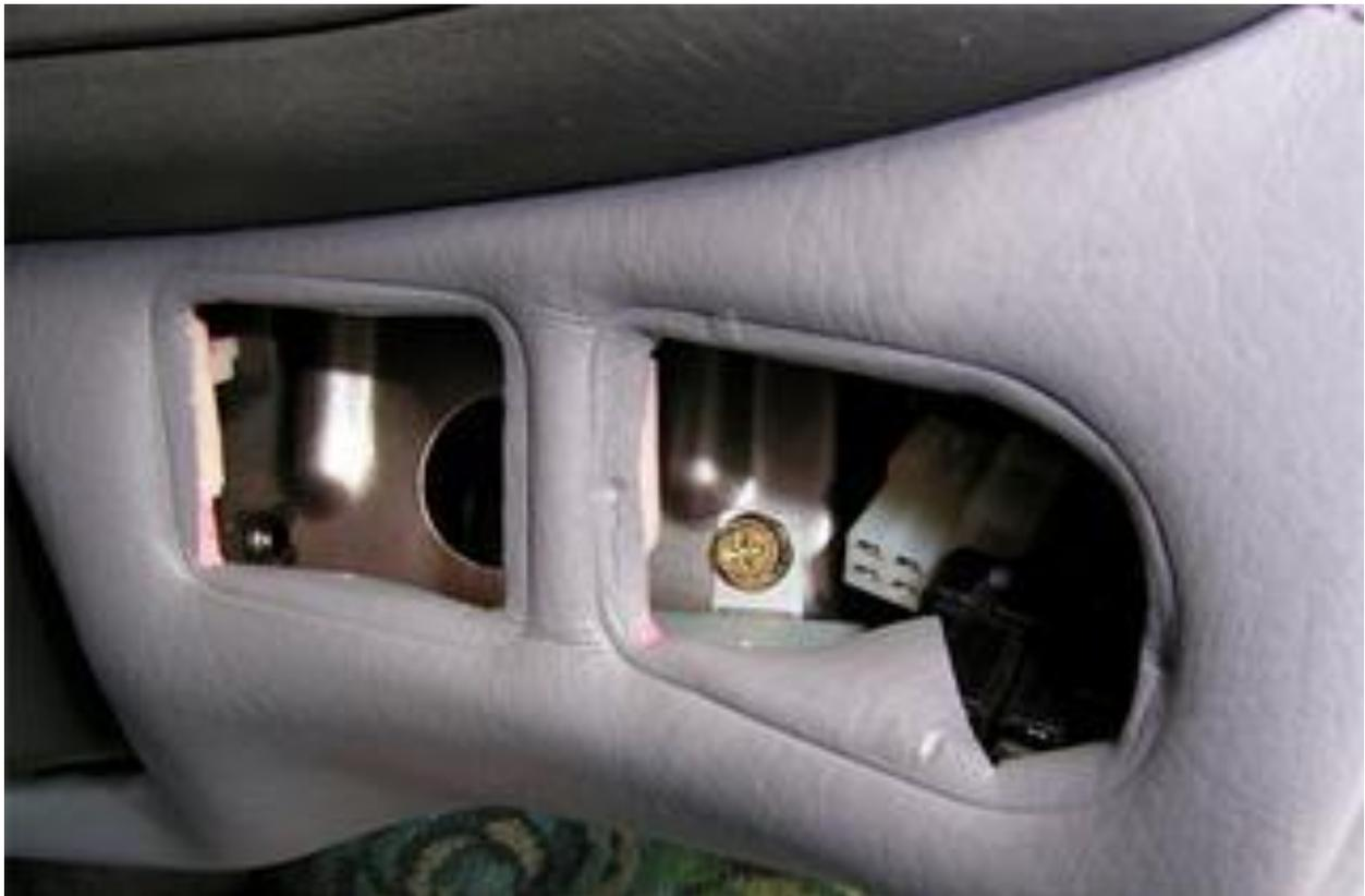
Get a mirror to see clip shape and position behind panel; place finger behind the opening and pull slightly upwards to unclip. NB: the clip is part of the fibreglass shell, do not break it!
