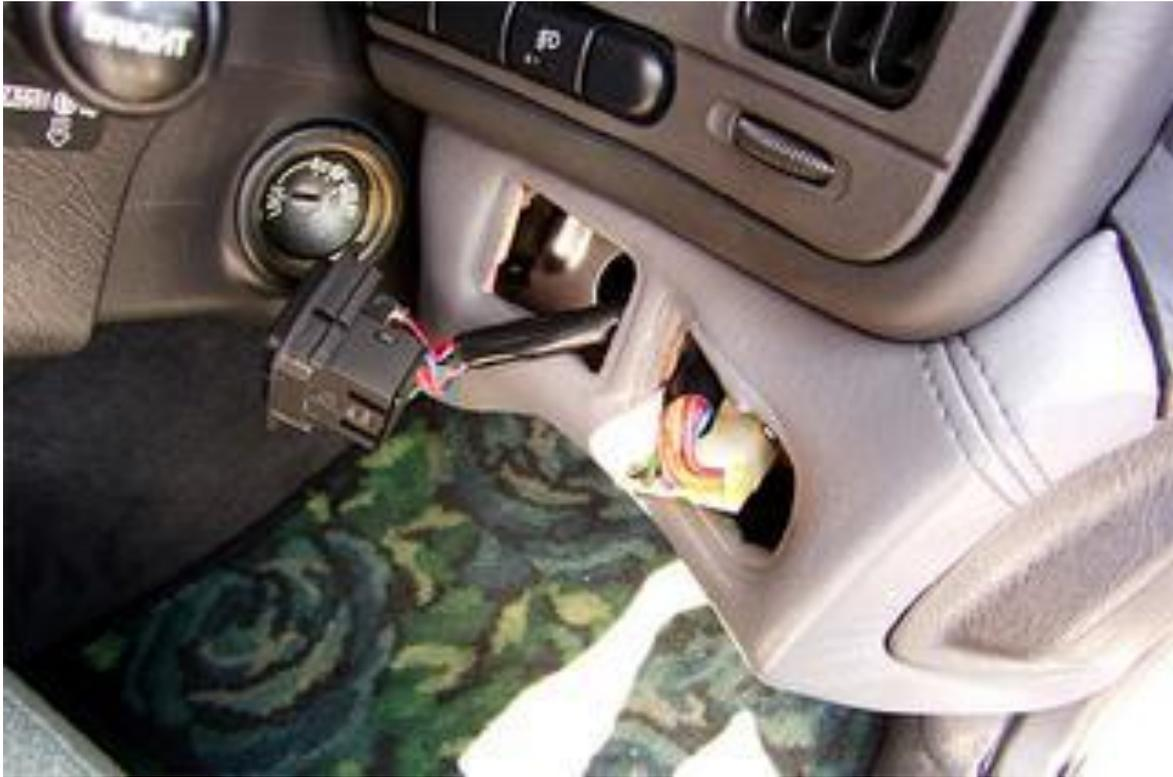
Remove the bolt that is exposed behind switches.
