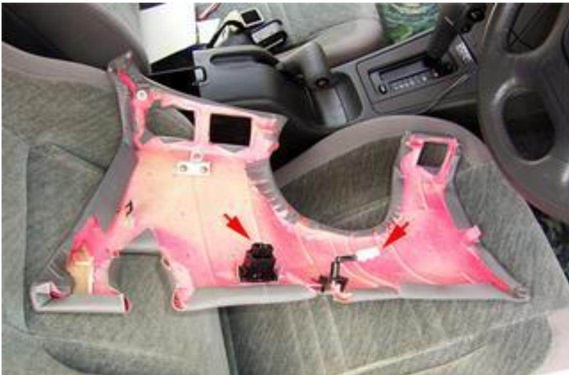
Next, slide fingers into the openings below the switch clusters and gently pull the switches forward.
