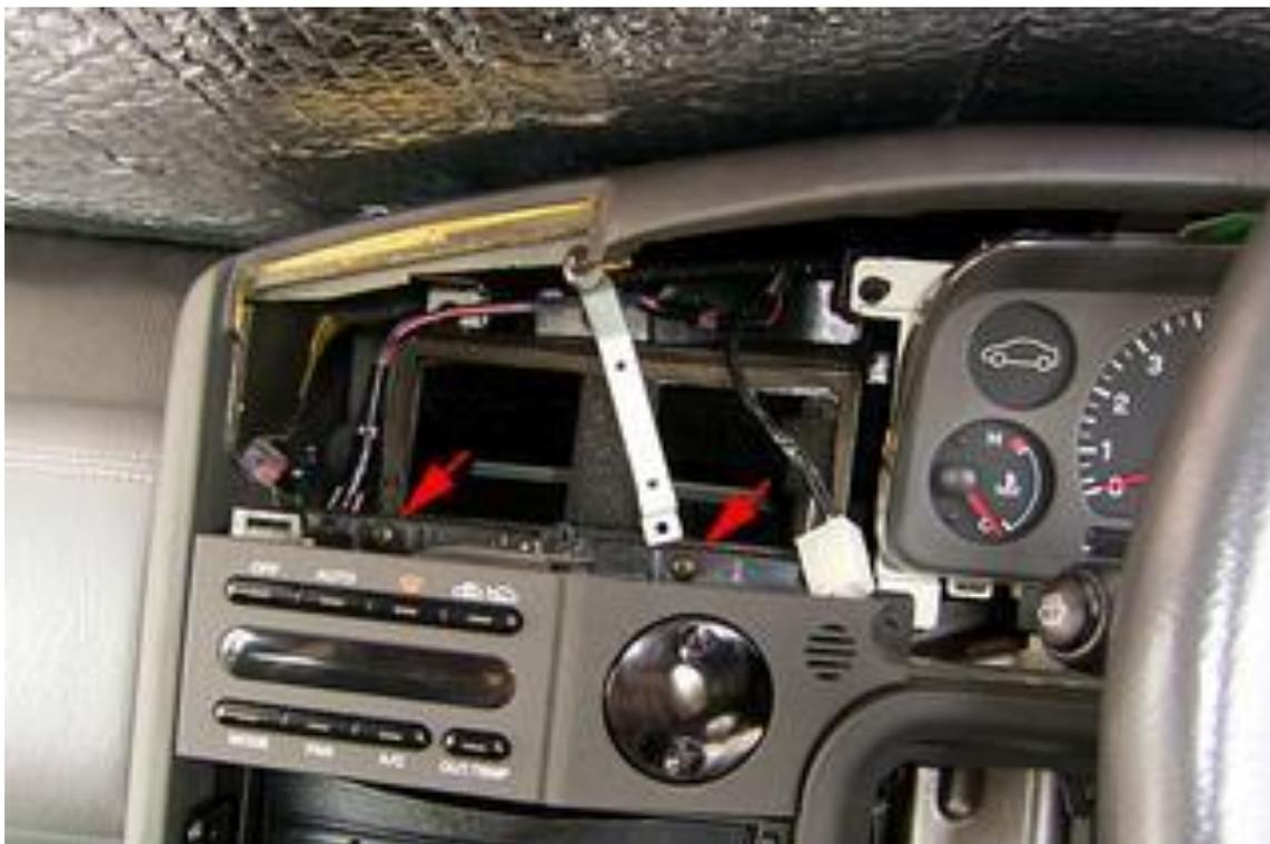
Remove the internal cover on the audio door using a fine flat blade screw driver for this - it has been documented elsewhere in this group ([maybe a link or additional photos](#)).
