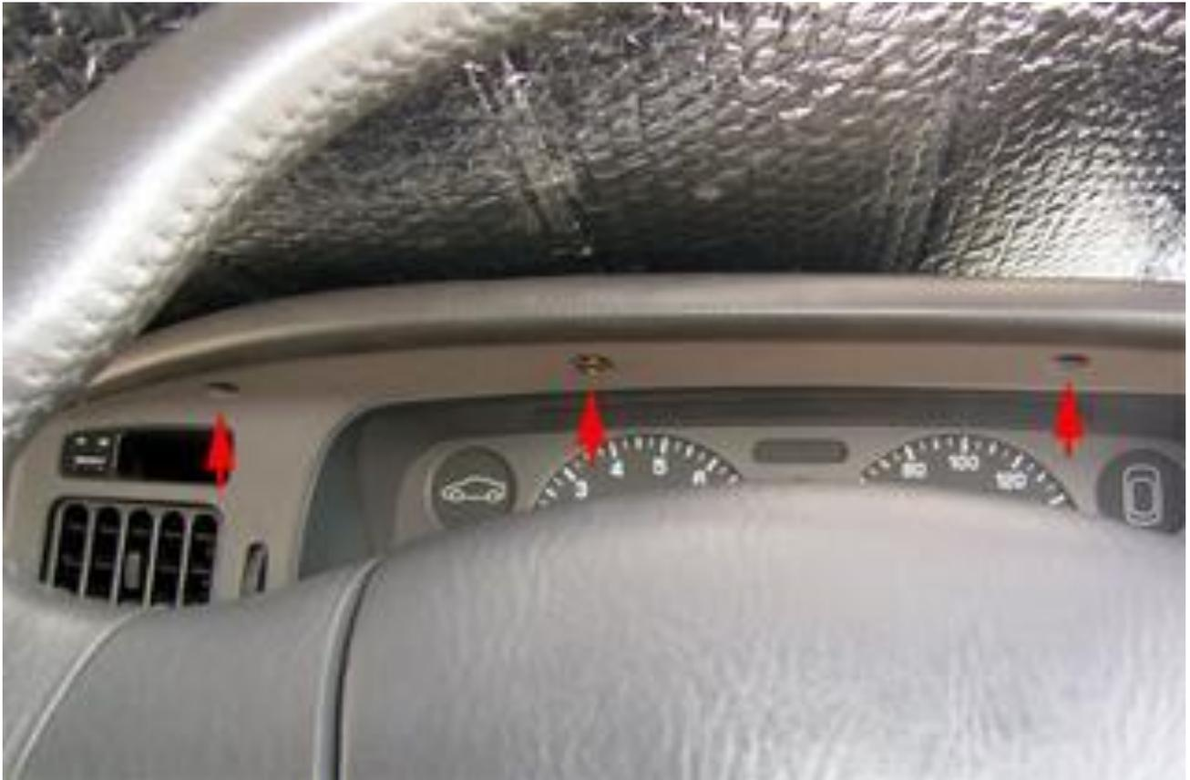
Pull the cluster surround forward, rest on steering rack cover while you unclip wiring connector from the clock.
