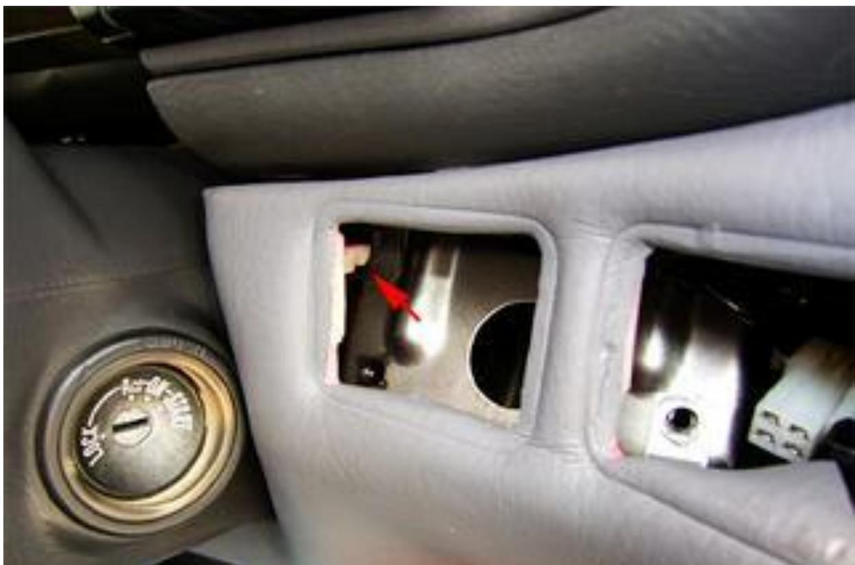
Under steering rack cover near 'Winter/Summer wipers switch' there is a small plastic screw that needs to be removed.
