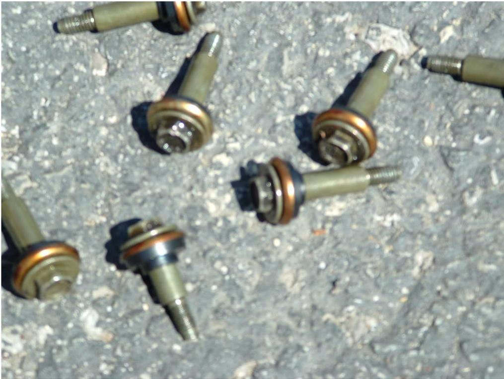
10) Carefully slide and maneuver the covers back into place and start bolting them back on with the 10 bolts per side. (The torque specs on these bolts are 10-14 ft-lbs).
