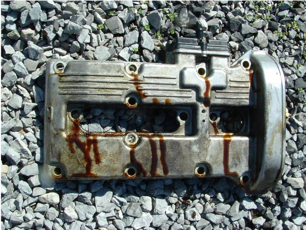
7) Take the actual valve cover over to a bench and remove the three rubber seals. They're relatively easy to remove (one goes all around and the other two go around the middle area where the coil packs sit).
