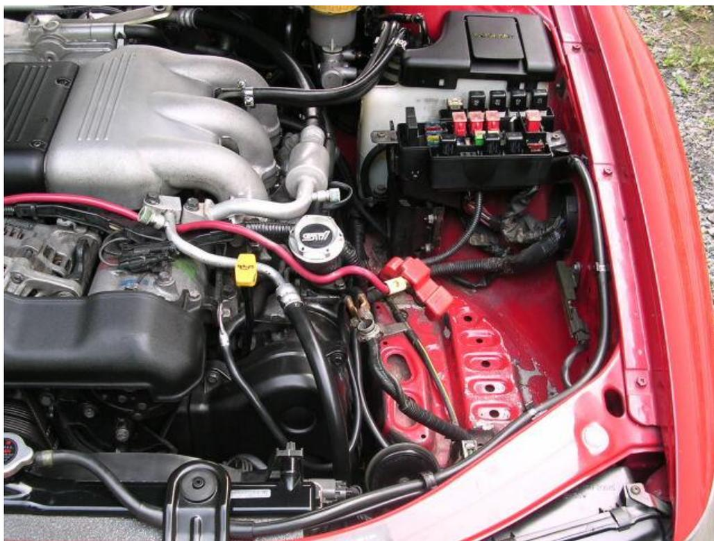
2) Unscrew the 2 clamps from the intake that goes onto the throttle body and MAF.
