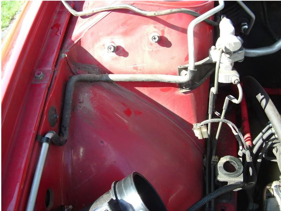
4) Unbolt the engine oil filler tube.
