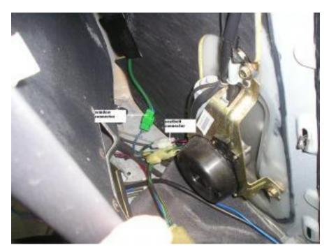
5. Switch the connections (make sure the feed end is connected to the motor). Remember, the connectors are the same type for both the window and the seatbelt motor so you can't make a mistake. 6. Try the switches before you close up everything.
