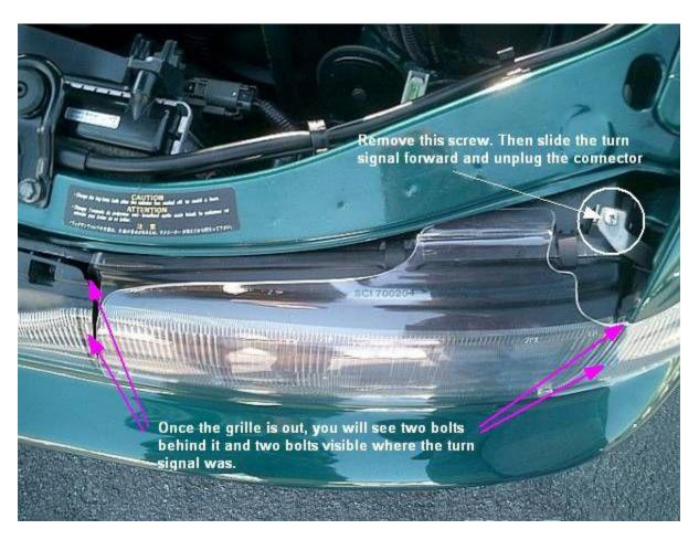
\*\*\*\* Be sure that the guide pin (shown below), goes into the hole in the fender when you reinstall the signal.
