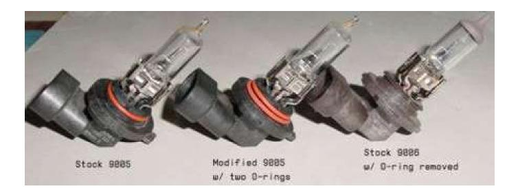
The picture above shows (left to right) the stock 9005, the modified 9005, and the stock capped 9006 bulb. Some think that an extra O-ring should be used (shown above) to insure a tight fit, but I have not had to do this.
