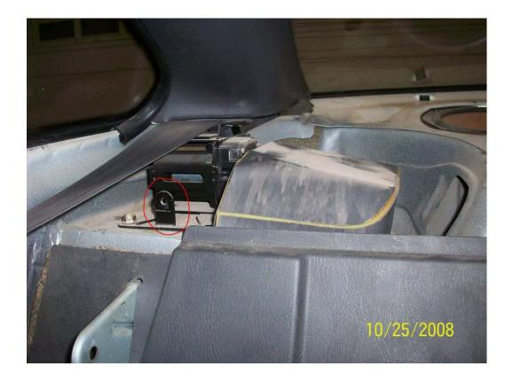
I removed the rear strut mounting bolt cover to expose the area a little more. The circled area is the screw that can only be removed after the side trim piece has been removed. Repeat for both sides of the rear seat.
