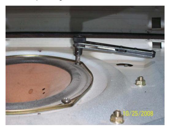
The new speakers simply bolt in place using the same screws. Mine are Pioneer 6x9s.
