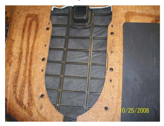
The finished product after trimming by using a box cutter knife:
