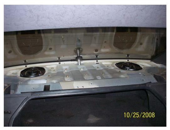
Turn the rear deck over and make sure that the outline of your speakers will fit inside the oem speaker area. I trimmed a little on the outside edges for the Pioneers.
