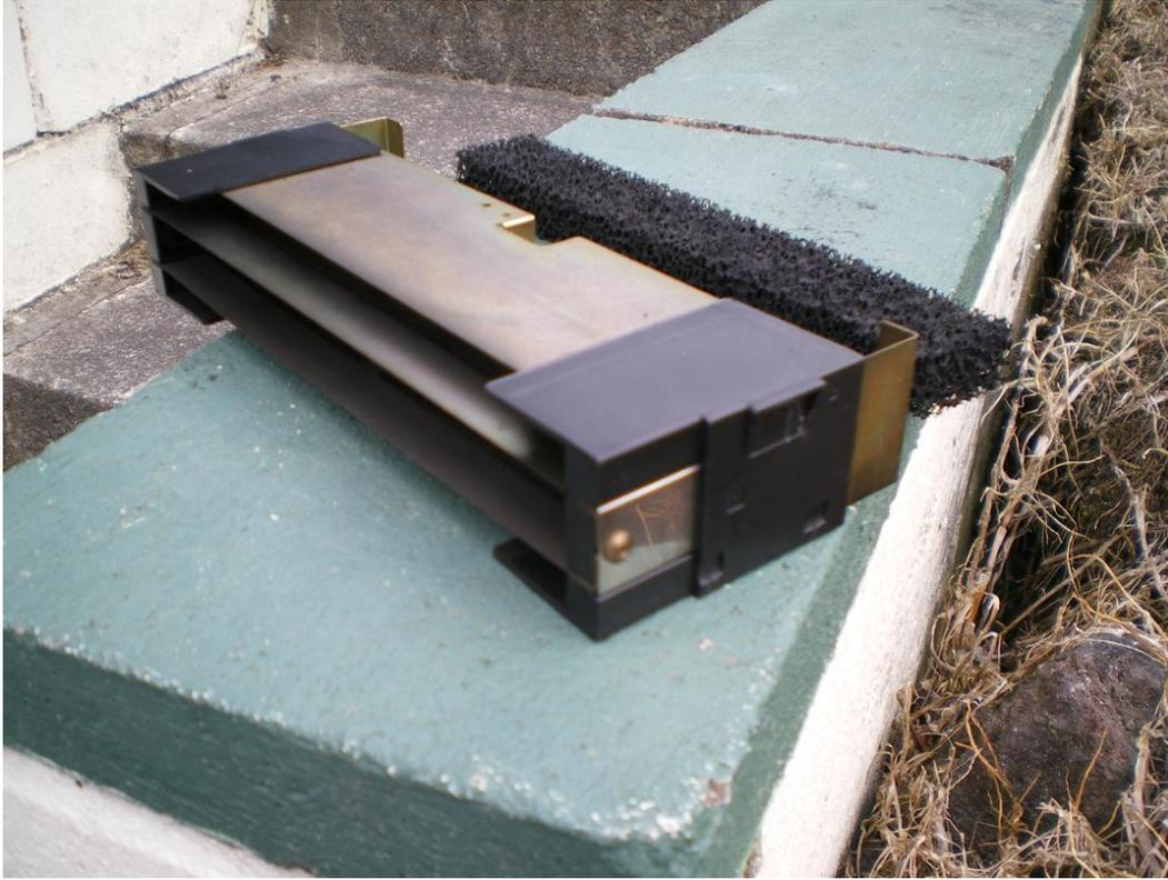
The outside plates are joined to form a shield. The inner plates are also joined and these are the High Voltage ones!!
