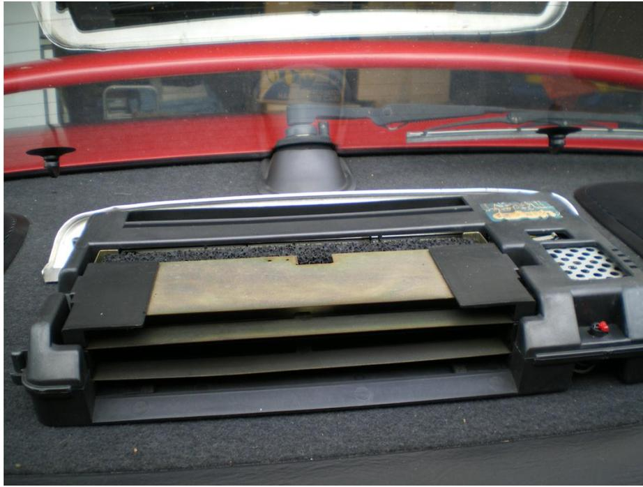
The charcoal filter is removed and the cutout in the gold pasivated metalwork is to allow fingers on each side of the filter for easy removal.
