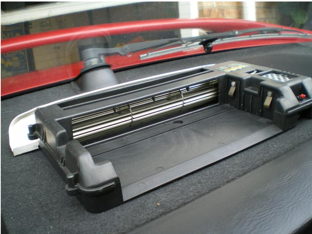
The high voltage plates & charcoal filter are out of the unit.
