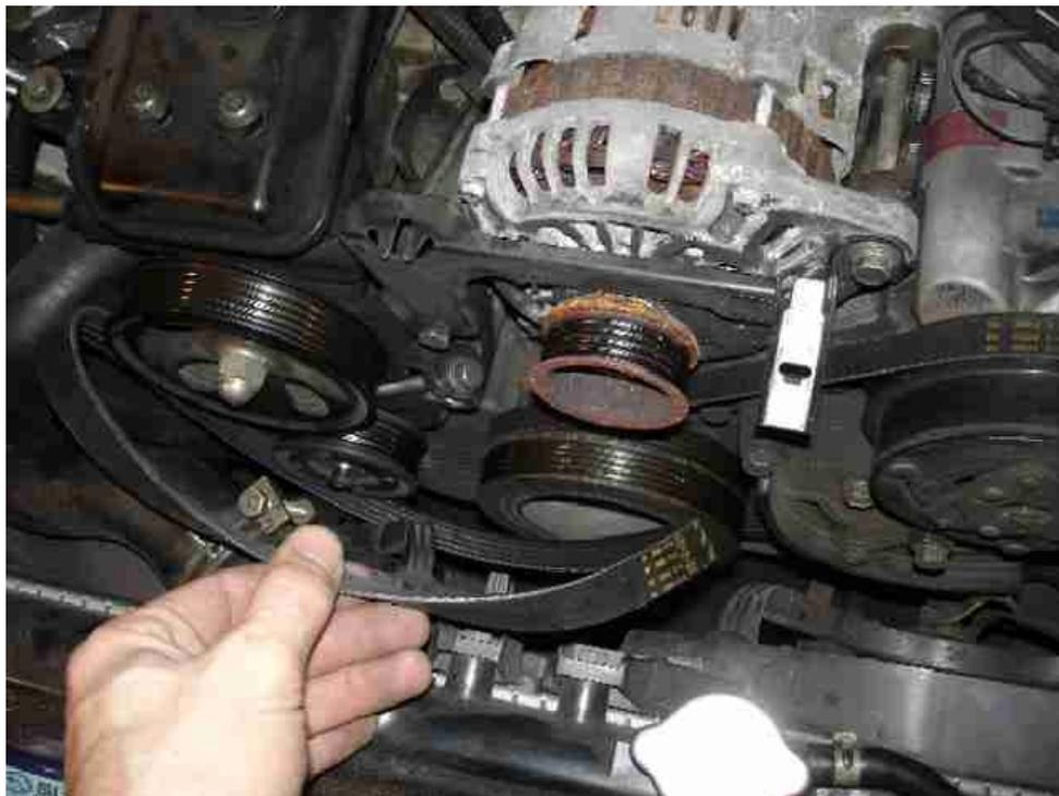
Tighten the tensioner pulley screw clockwise.
