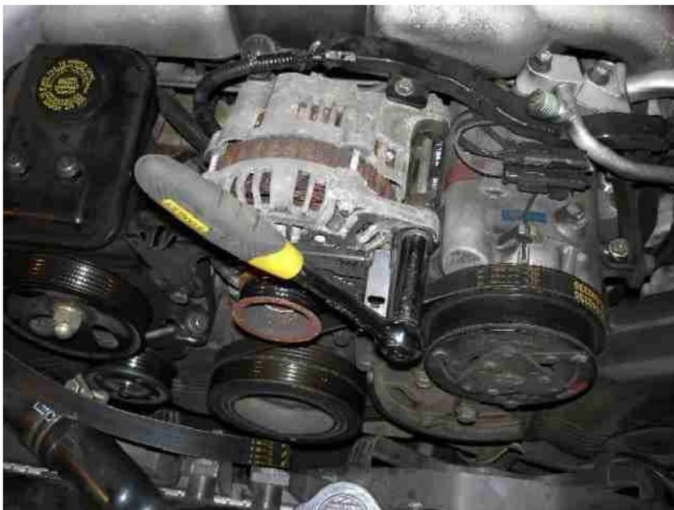
Install the lower alternator screw. Tighten it and also tighten the upper pivot screw.
