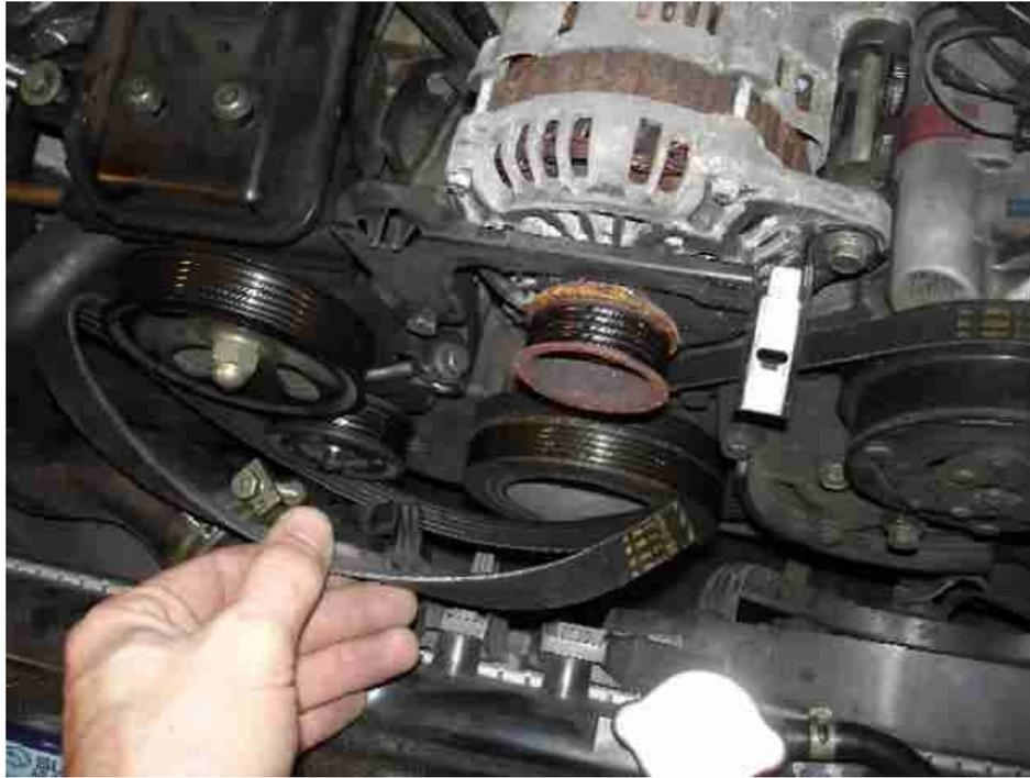
Remove the charging cable and unplug the indicator / exciter plug from the side of the alternator. Be sure that the battery ground cable is disconnected before doing this step.
