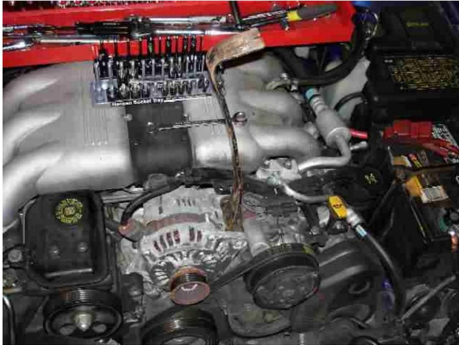
The alternator lifted from the mounting location.
