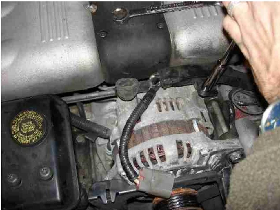
Secure the charging cable to the lug on the alternator. Reattach the battery ground cable.
