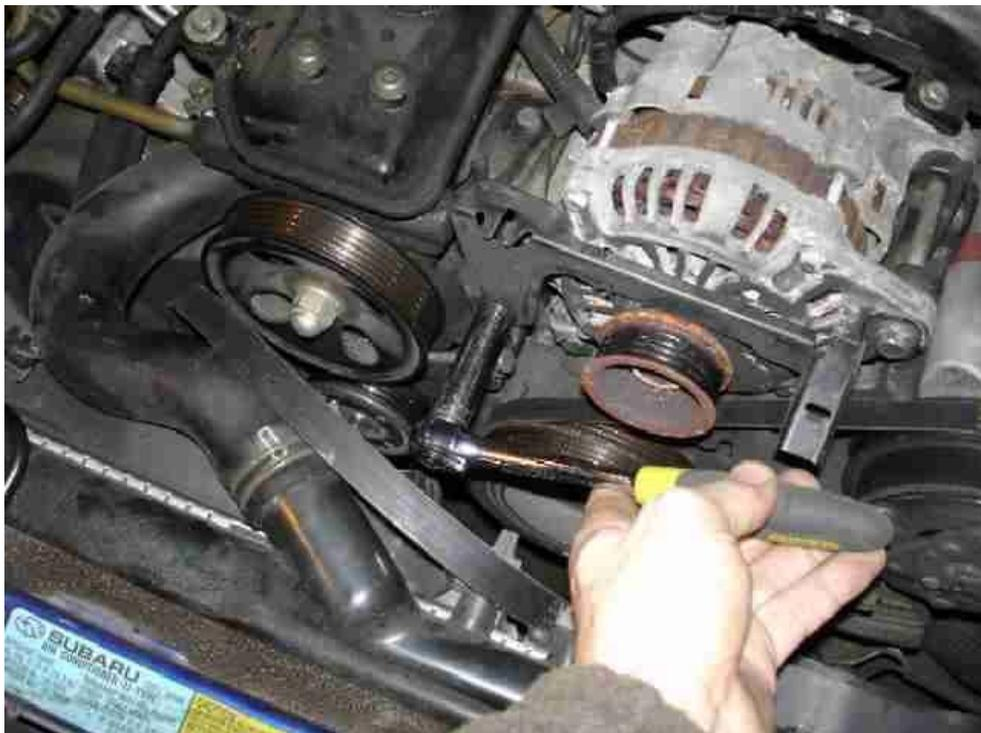
Remove the upper alternator pivot and bracket screw.
