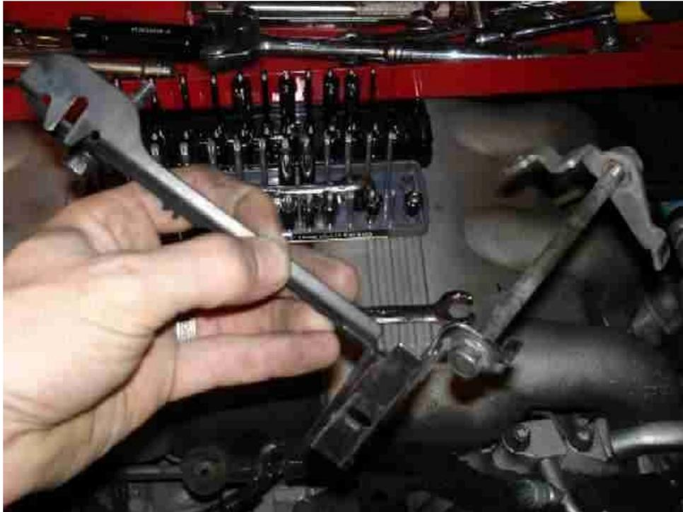
Install the upper alternator pivot screw. Leave it loose at this time.
