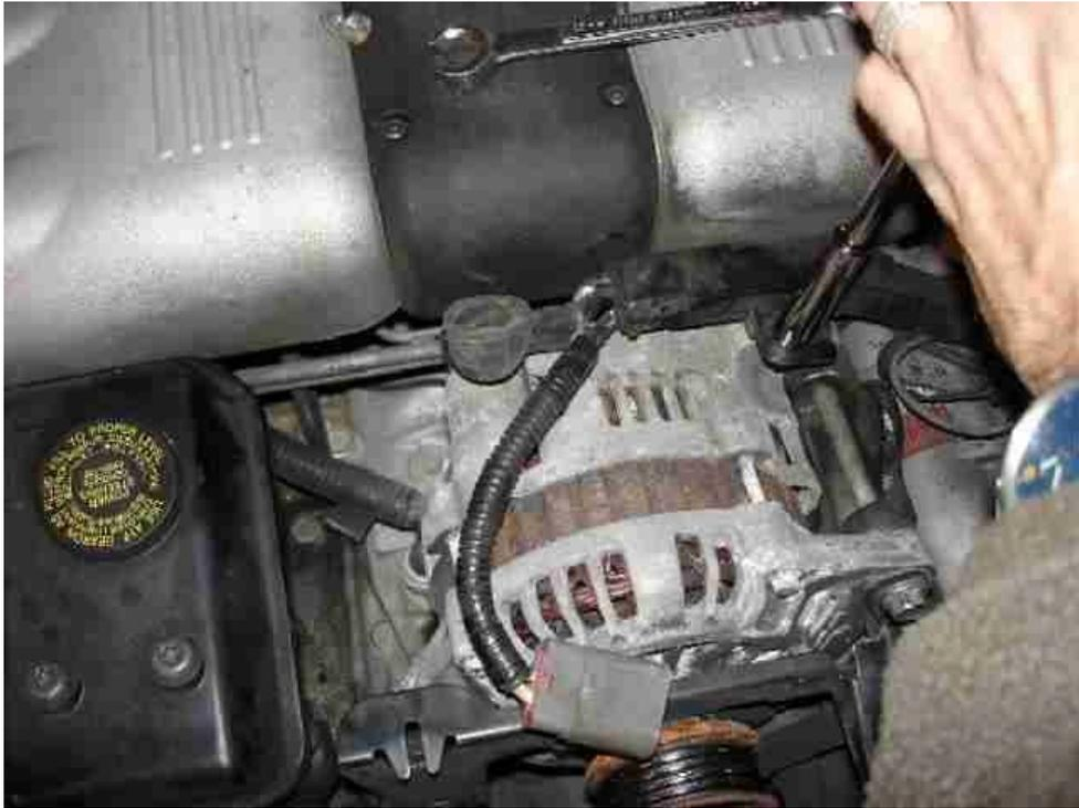
Remove the lower alternator and bracket screw.
