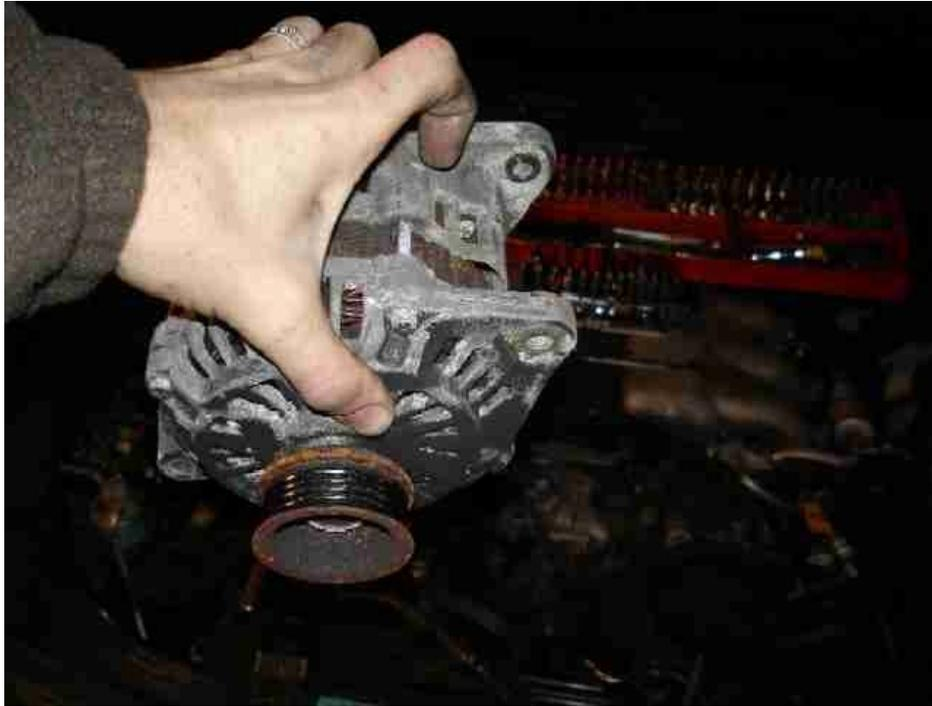
Careful use of a pry-bar and hammer are the best tools for getting this to fit back into the mounting area.
