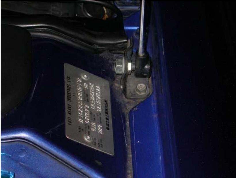
Locate the spot on the hood where the factory lifters would go (you should see a spot on the hood from the mold where the lifters would go) drill a hole the size of the shank of the ball studs.
