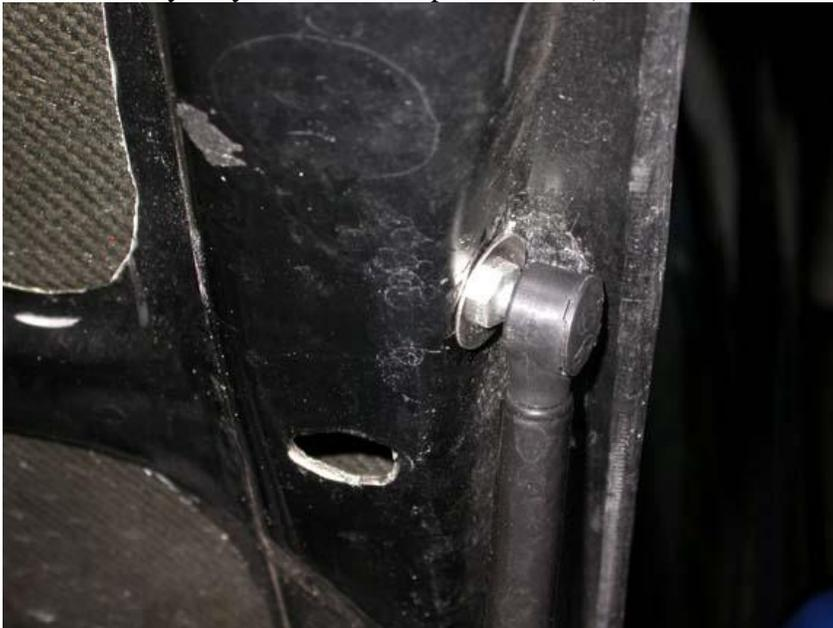
3. Install the ball stud into the hood with the fender washer on the outside and the nut on the inside of the hood. (If you can put a washer or locknut on the inside of the nut for more support)
