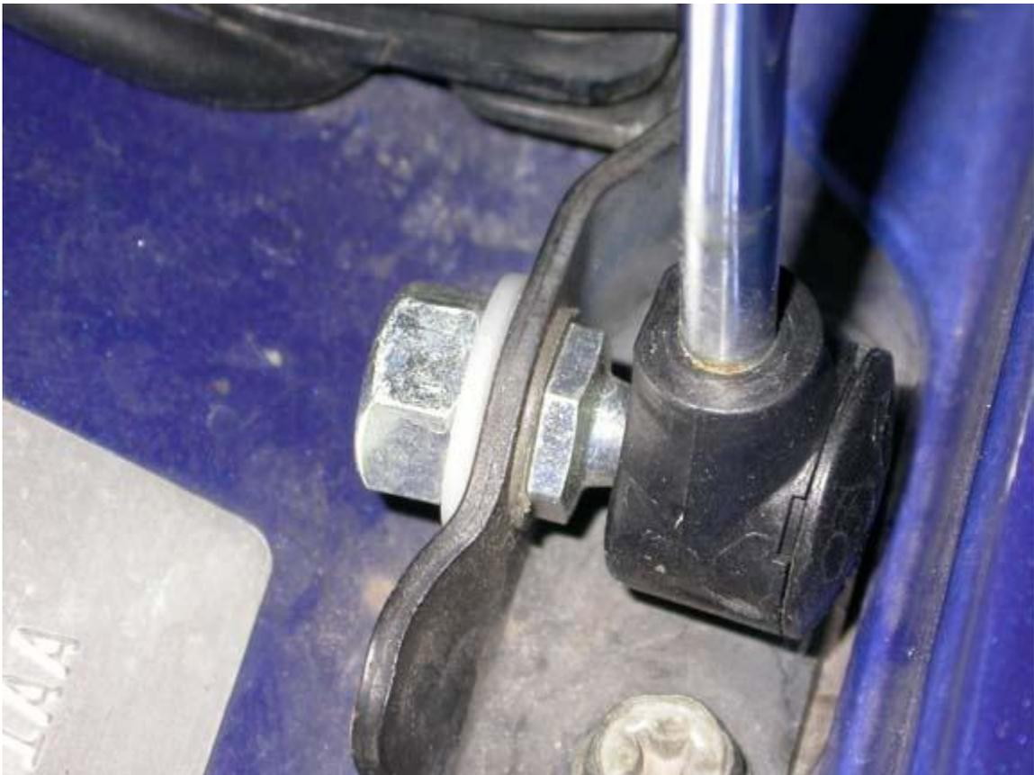
3. Install bracket and ball stud assemble on to car. (Use the factory bolts)
