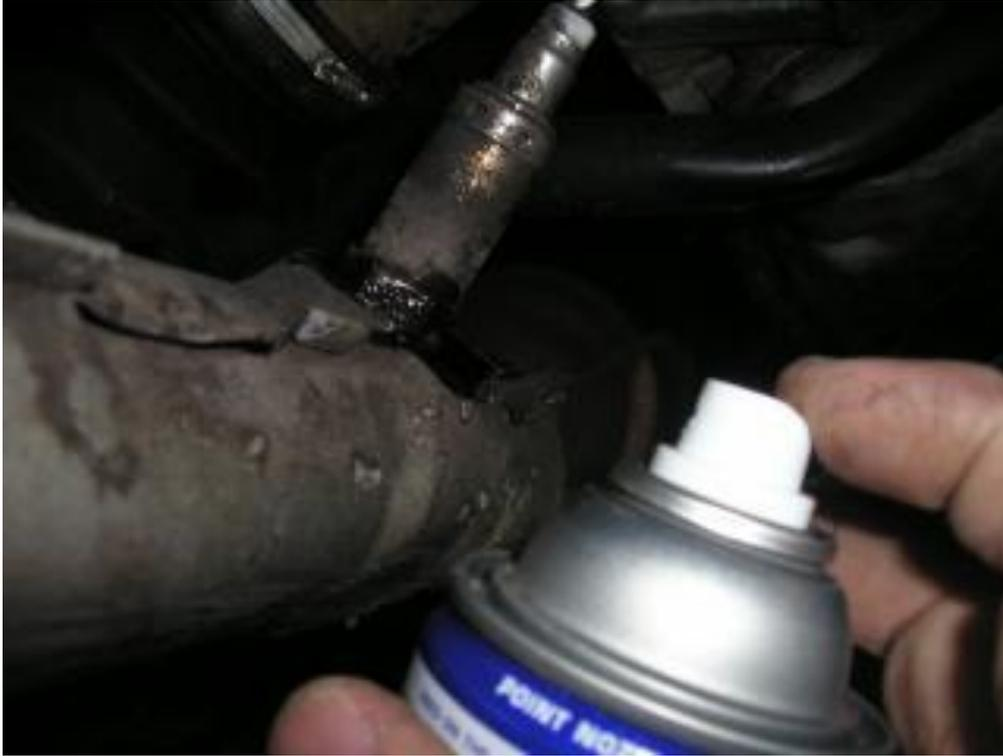
5. Use a box wrench, open end wrench or a special socket for Oxygen sensors (I used the special socket with a 1 inch box wrench).
