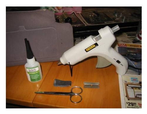
Seal the cut in the visor fabric with hot glue.
