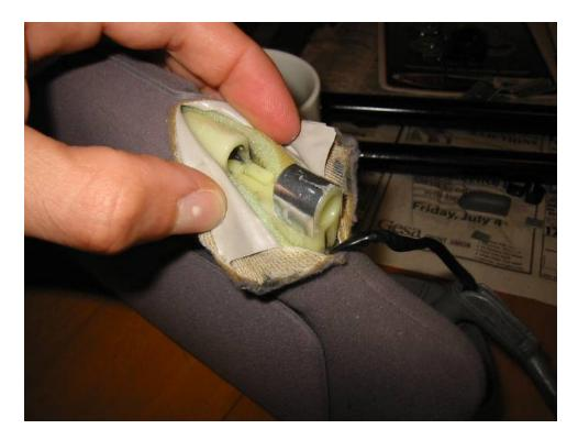
My first attempt to fix the break was with superglue and a strip of aluminum can. I roughened the visor plastic and the strip with emery cloth, and the superglue held well enough, but the AI snapped the first time I tried to rotate the visor down. When that happened, I realized that the plastic loop in the visor supports a very large stress, and I was no longer surprised that the plastic eventually failed.
