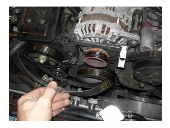
Tighten the tensioner pulley screw clockwise.
