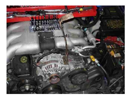
The alternator lifted from the mounting location.
