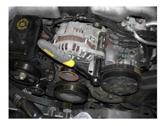
Install the lower alternator screw. Tighten it and also tighten the upper pivot screw.
