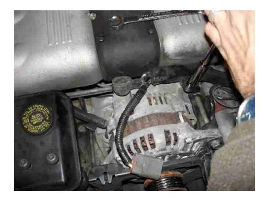
Remove the lower alternator and bracket screw.
