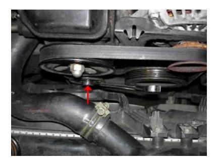
Loosen the tensioner adjustment screw counter-clockwise (socket wrench is on it below).
